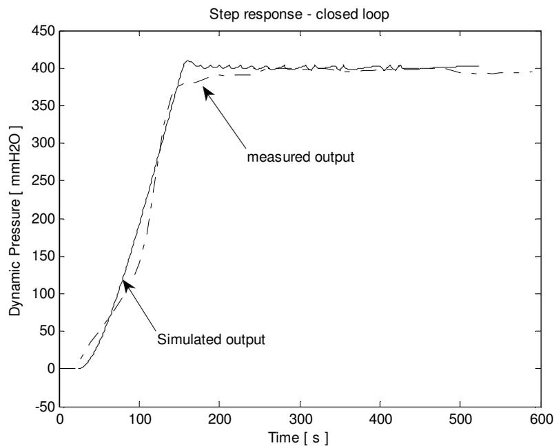
Figure 6. Step response : measured and simulated.
