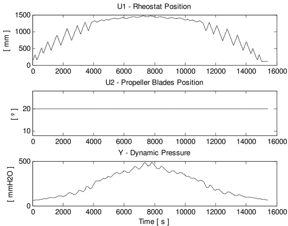
Figure 2. Input and output signals for identification n° 1.
