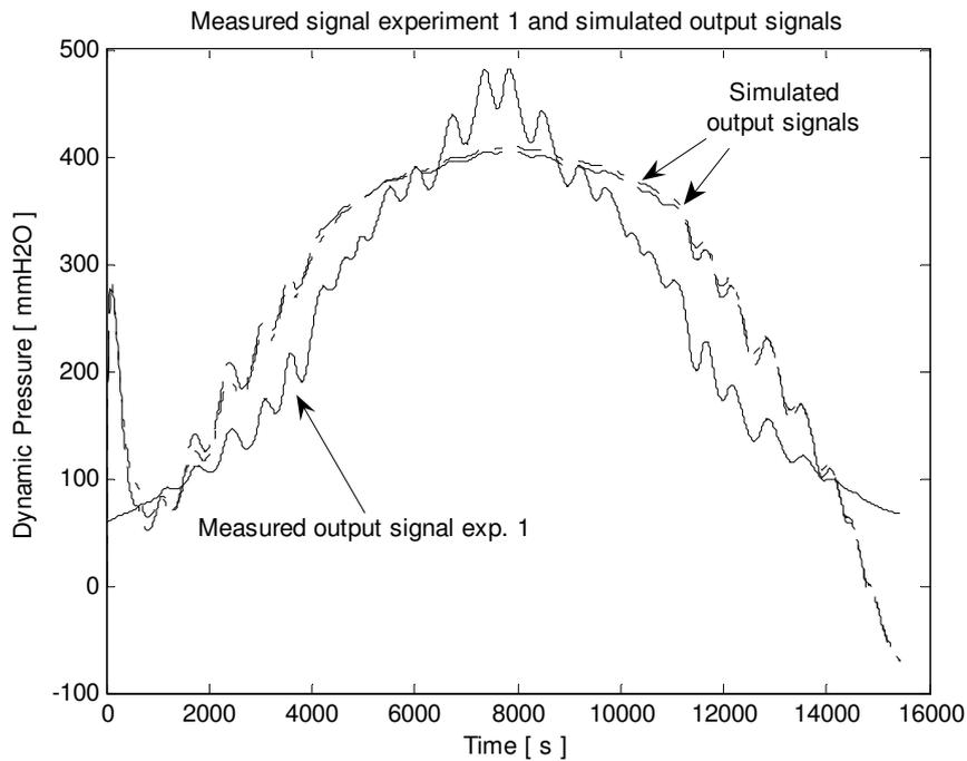
Figure 5. Measured and predicted outputs for the input used in experiment n° 1.
