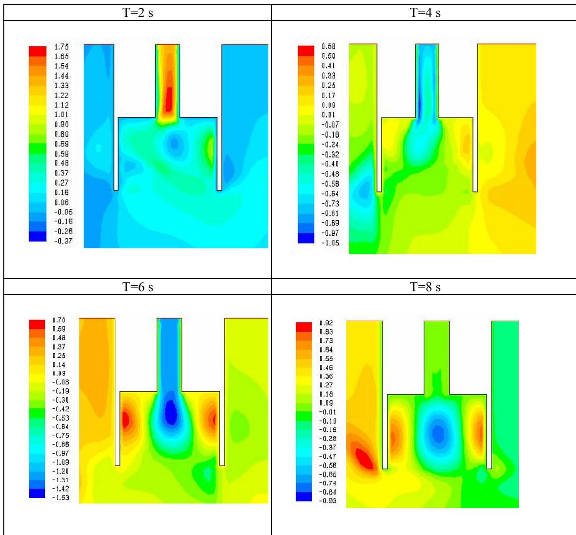
Figure 10. Velocity field of the VOF methodology (m/s)
