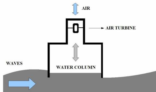
Figure 1. Oscillating water column system.
