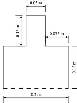
Figure 2. Oscillating water column chamber.
