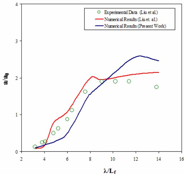
Figure 6. Relative wave amplitude distribution with the wave length ratio variation.
