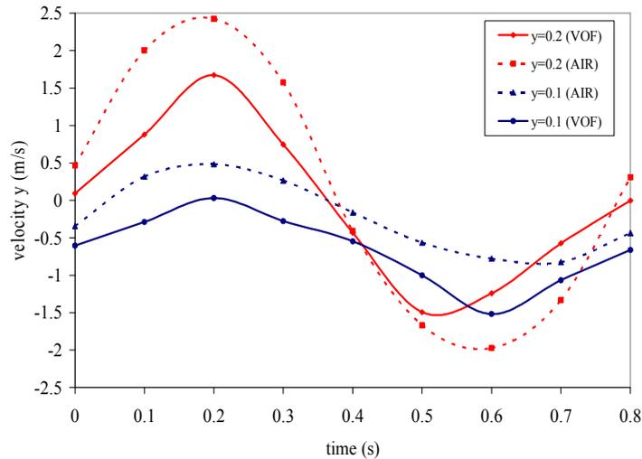
Figure 8. Vertical velocity comparison in OWC chamber.
