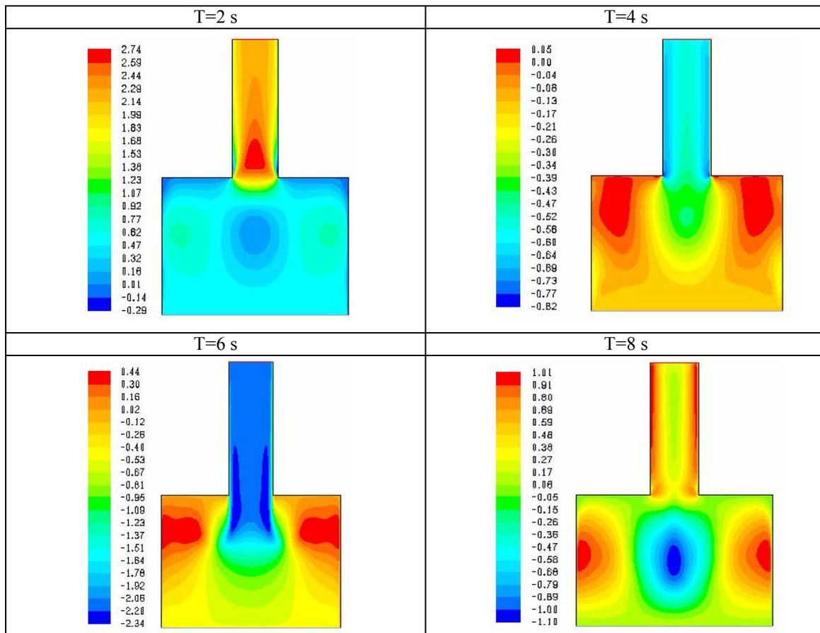
Figure 9. Velocity field of the AIR methodology (m/s)
