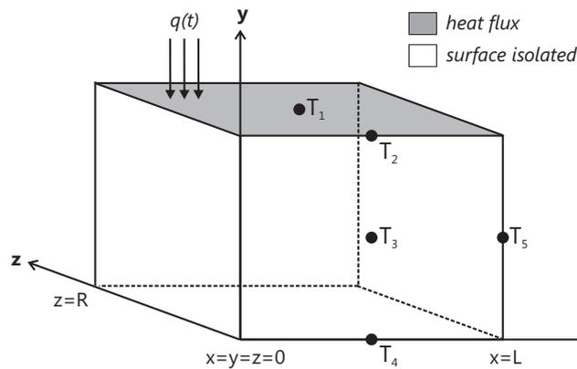
Figure 3. Schematic of a rectangular solid with heated superior surface and all other surfaces isolated with locations of positions used for comparison.
