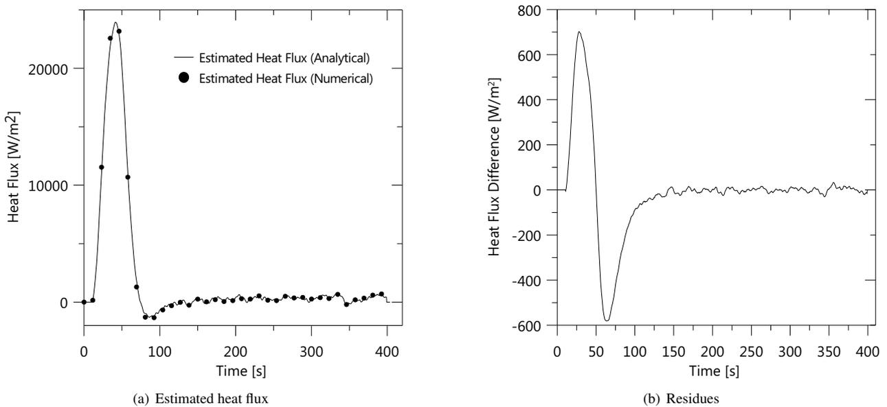
Figure 5. Heat flux for a cast iron sample
