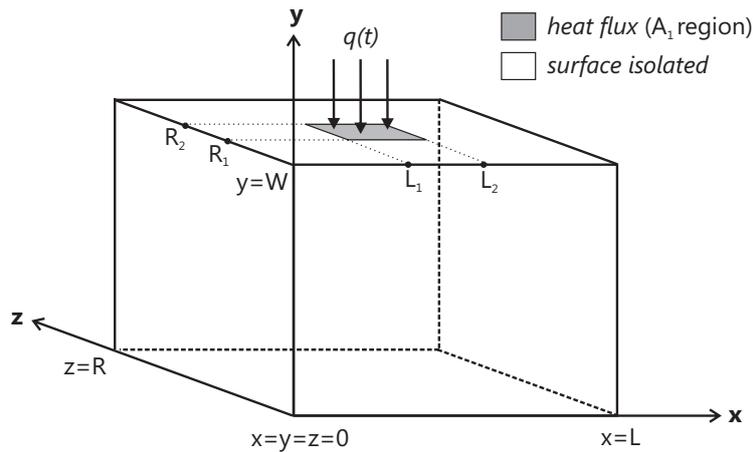
Figure 1. Equivalent three-dimensional transient thermal model
