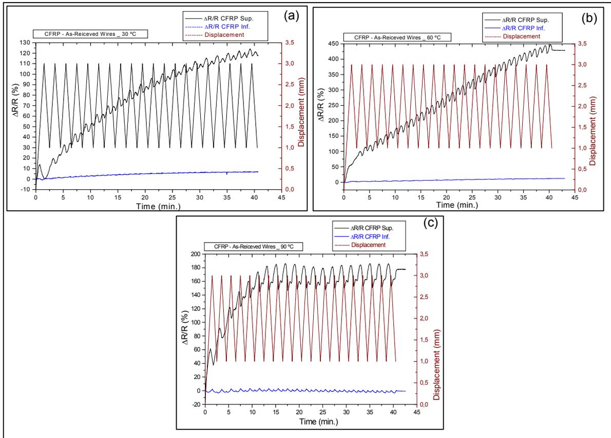
Figure 7. Behavior of  $\Delta R/R$  for the superior and inferior layers and displacement in function of the time for the composites with as-received NiTi wires: 30 °C (a), 60 °C (b) and 90 °C (c)
