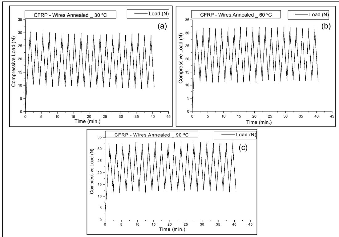
Figure 11. Evolution of the mechanical loading during the cycling of CFRP with annealed NiTi wires: 30°C (a), 60°C (b) and 90°C (c)
