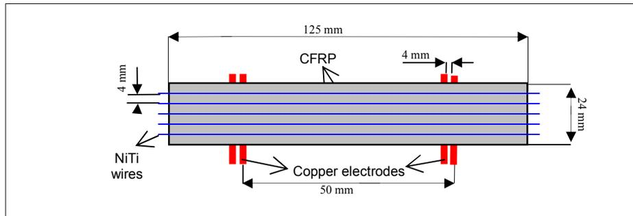
Figure 1. Schematic drawing of the CFRP-NiTi active composite
