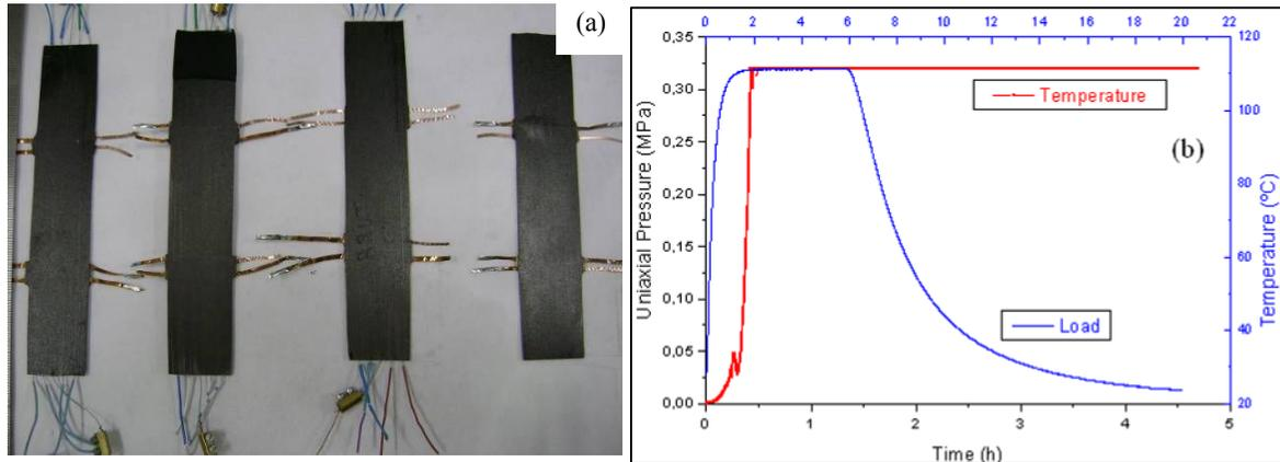
Figure 3. CFRP-NiTi active composites (a) and cure cycle (b)
