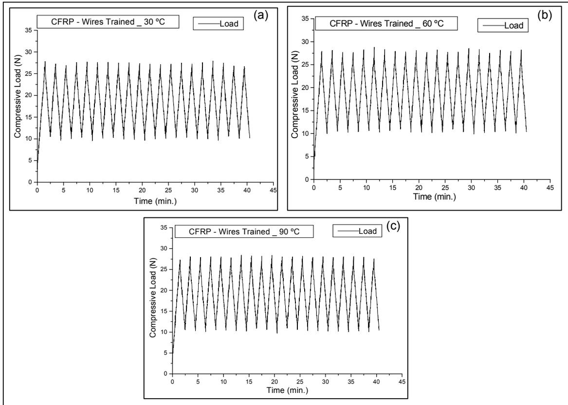
Figure 12. Evolution of the mechanical loading during the cycling of CFRP with trained NiTi wires: 30°C (a), 60°C (b) and 90°C (c).
