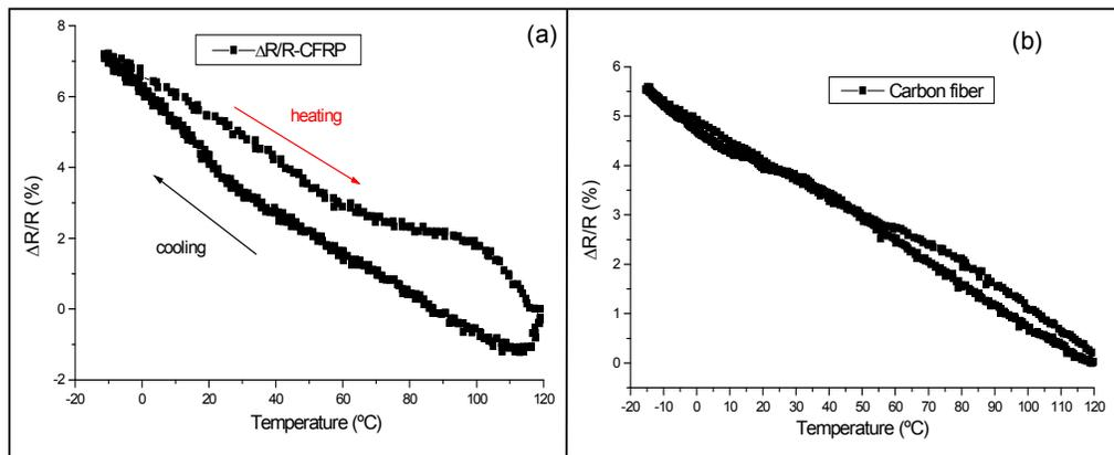
Figure 5. Electrical resistance change in function of temperature for the CFRP (a) and pure carbon fibers (b)
