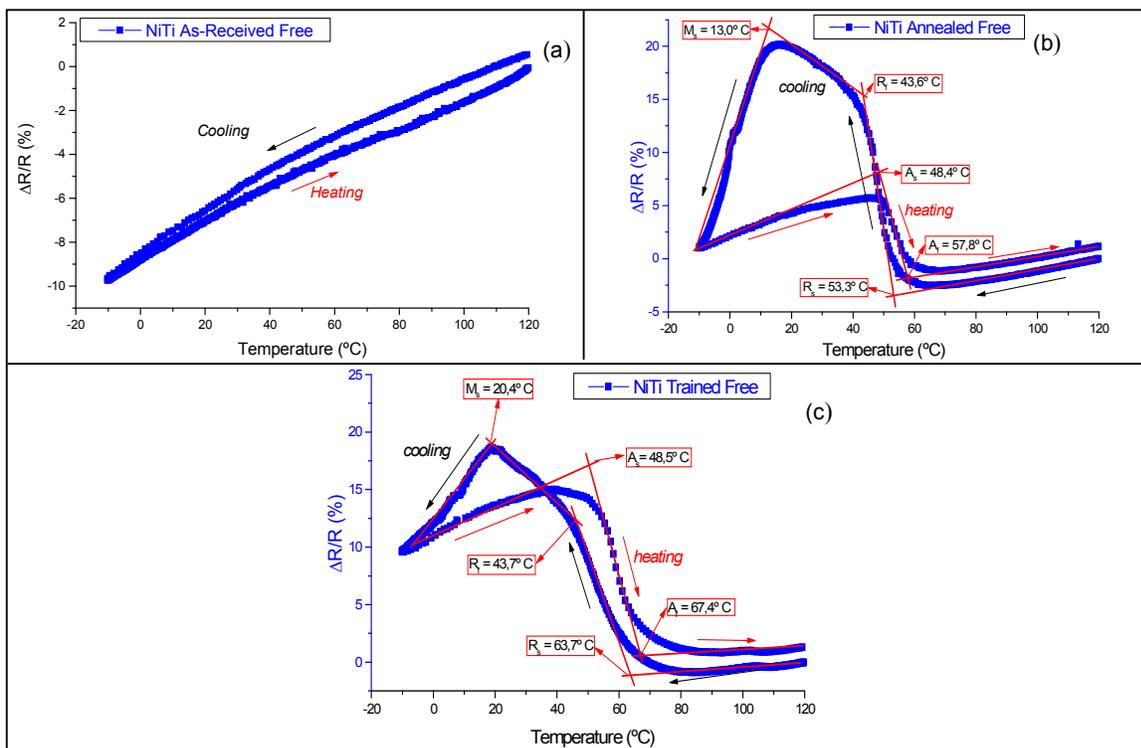
Figure 4. Electrical resistance change in function of the temperature for the NiTi wires: as-received (a), annealed (b) and trained (c)
