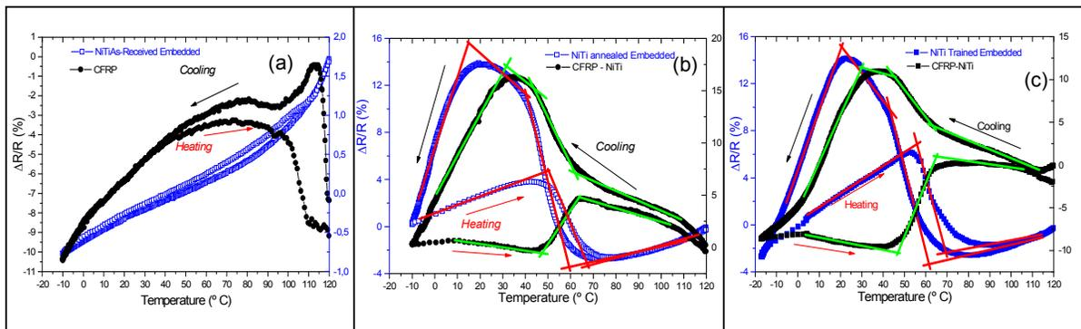
Figure 6. Electrical resistance change in function of temperature for the CFRP composites with NiTi wires in the following conditions: as-received (a) annealed (b) and trained (c)
