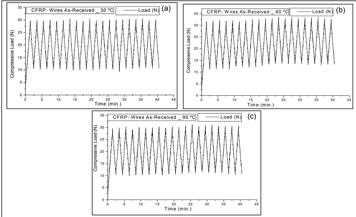
Figure 10. Evolution of the mechanical loading during the cycling of CFRP with as-received NiTi wires: 30°C (a), 60°C (b) and 90°C (c)
