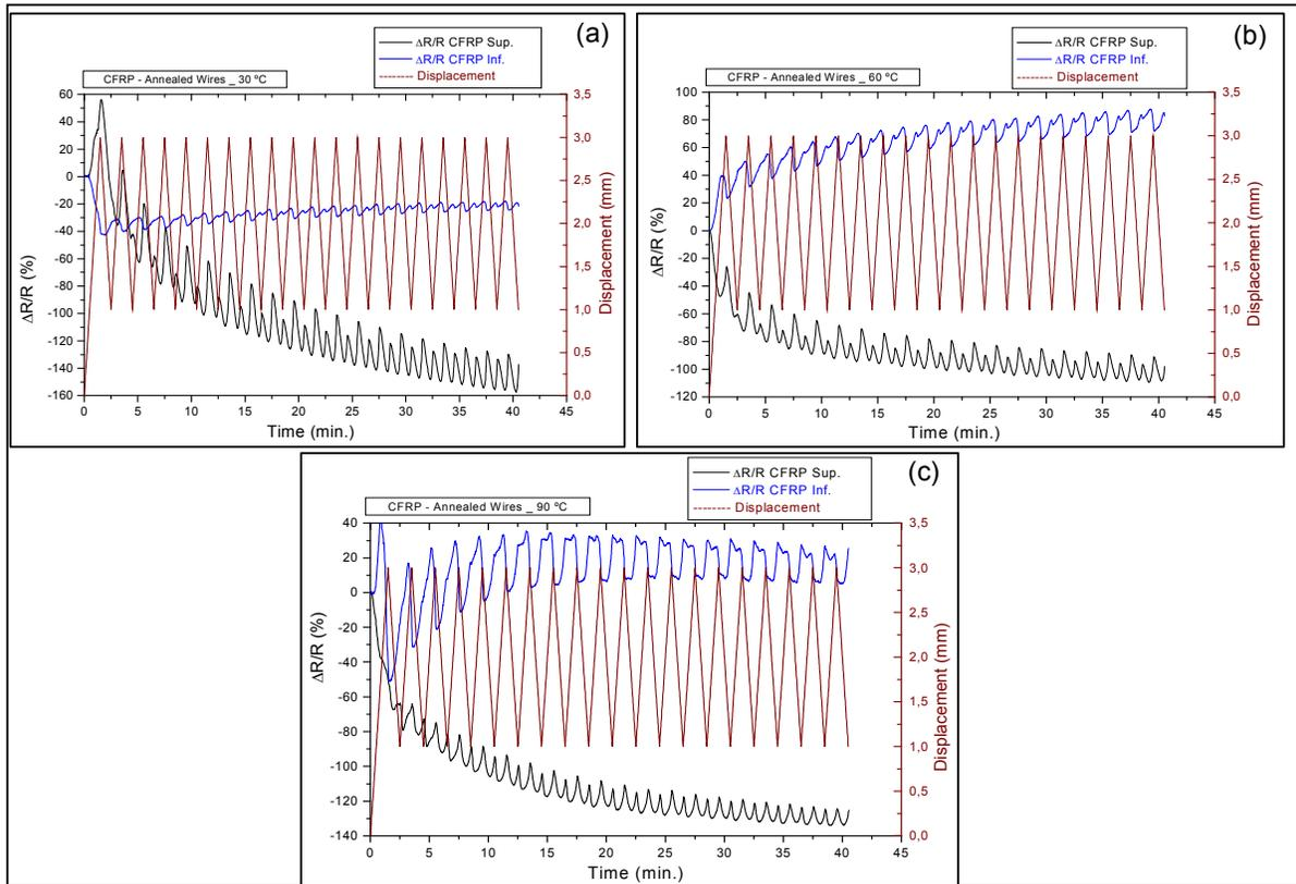
Figure 8. Behavior of  $\Delta R/R$  for the superior and inferior layers and displacement in function of the time for the composites with annealed NiTi wires: 30 °C (a), 60 °C (b) and 90 °C (c)
