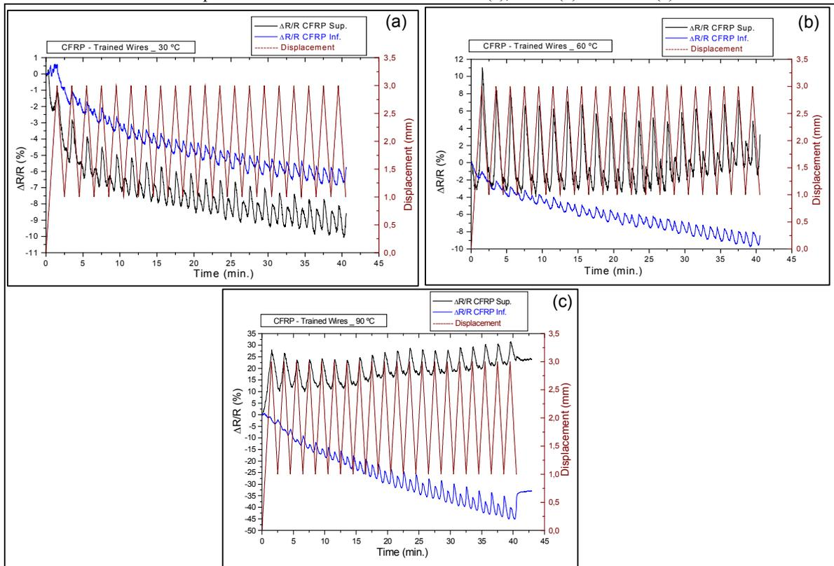
Figure 9. Behavior of  $\Delta R/R$  for the superior and inferior layers and displacement in function of the time for the composites with trained NiTi wires: 30 °C (a), 60 °C (b) and 90 °C (c)
