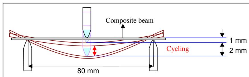
Figure 2. Schematic drawing of three points bending cycles in CFRP-NiTi active composites
