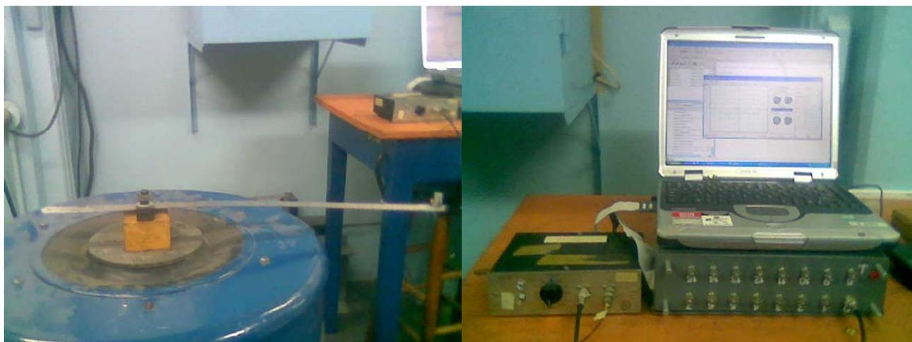
Figure 2. Instrumented beam and equipments used for data acquisition.
