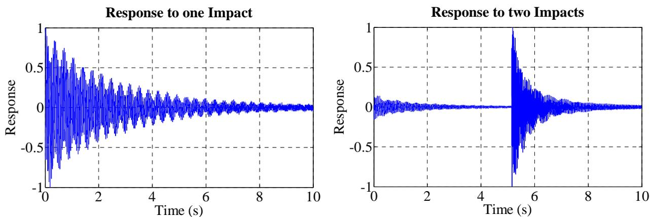
Figure 3. Response of the beam subjected to impact loads.
