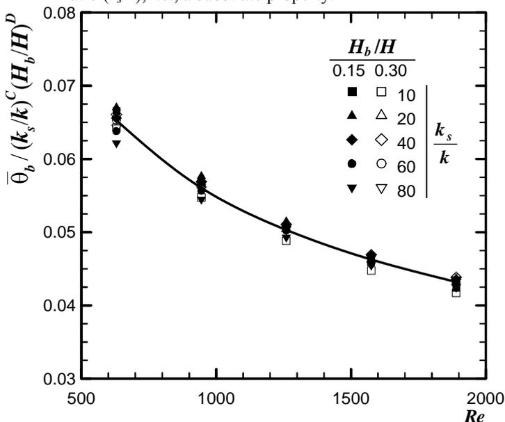
Figure 12. Dimensionless heater mean surface temperature rise above  $T_0$ .
