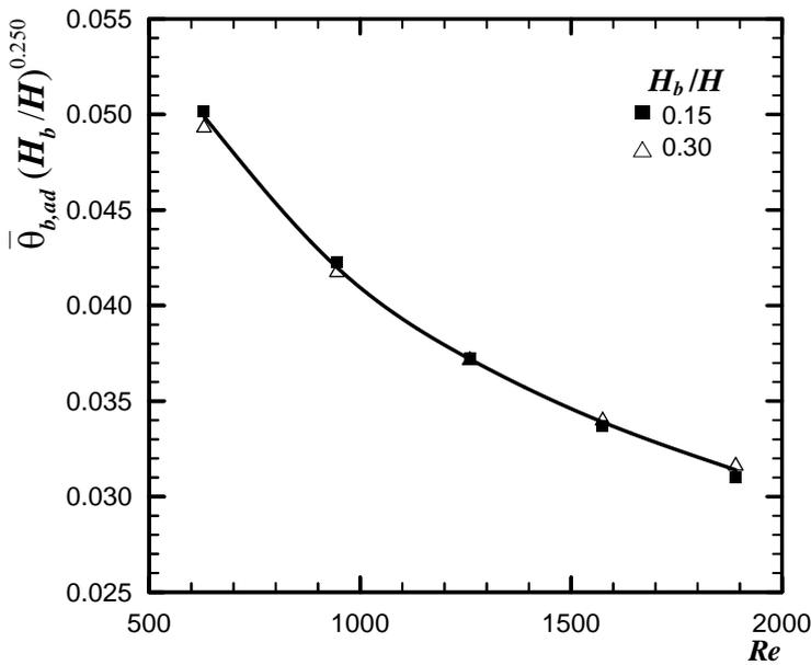
Figure 2. Heater dimensionless average adiabatic surface temperature.
