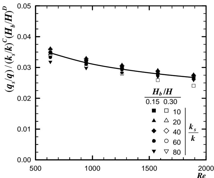
Figure 8. Fraction of ( $q_s/q$ ) conducted through the substrate plate.
