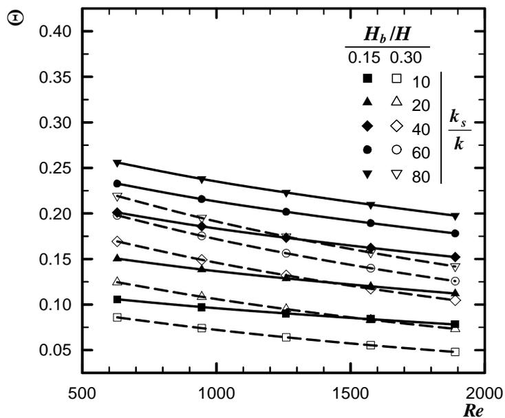
Figure 11. The adiabatic temperature rise due to upstream conduction.
