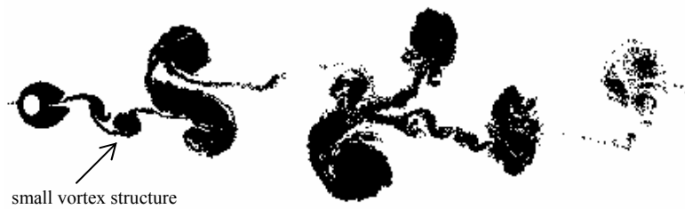
Figure 6. Mode of vortex formation for circular cylinder vibration, for A/d = 0.5 , St_b = 0.064 and Re=1.0 \times 10^5 .
