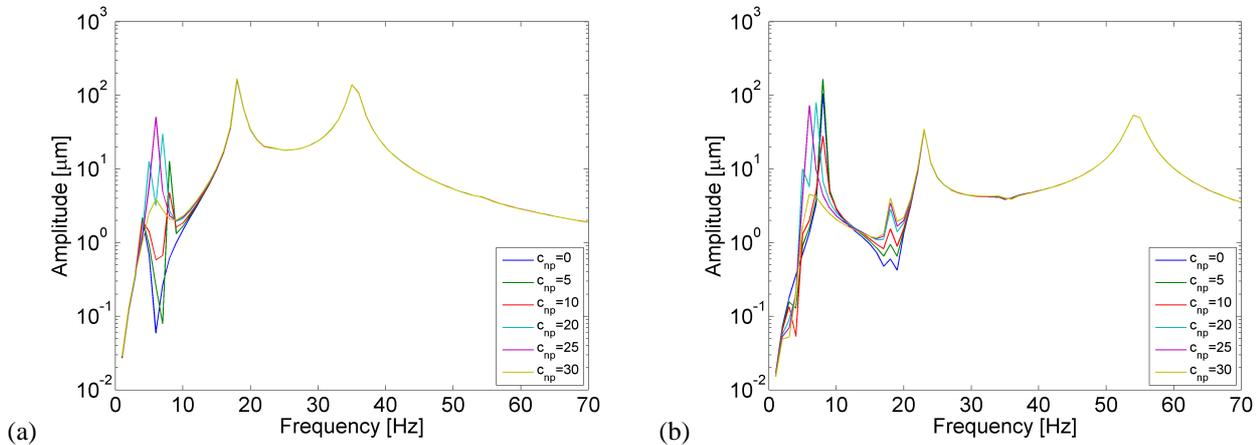
Fig. 6: Bearing case vibration amplitude (a – direction Y; b – direction Z) with modes 1 and 2 coupling.
