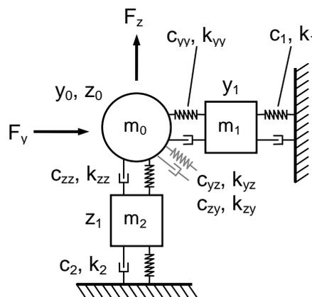
Fig. 2: Theoretical foundation structure (Okabe and Cavalca, 2008).
