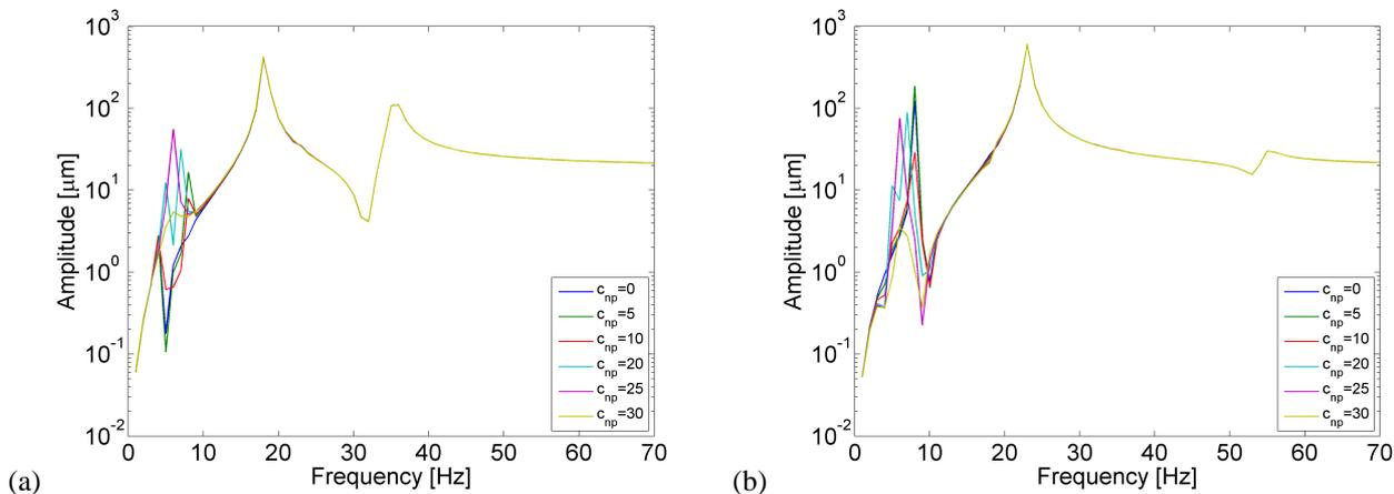
Fig. 4: Disk vibration amplitude (a – direction Y; b – direction Z) with coupling of modes 1 and 2.
