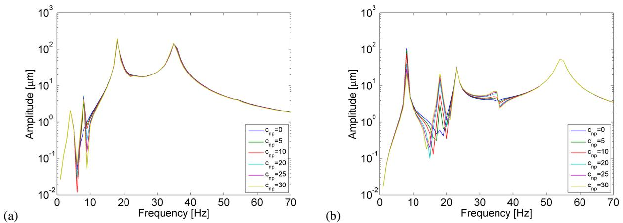
Fig. 9: Bearing case vibration amplitude (a – direction Y; b – direction Z) with modes 2 and 3 coupling.
