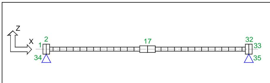
Figure 1: Finite element model of the rotor.
