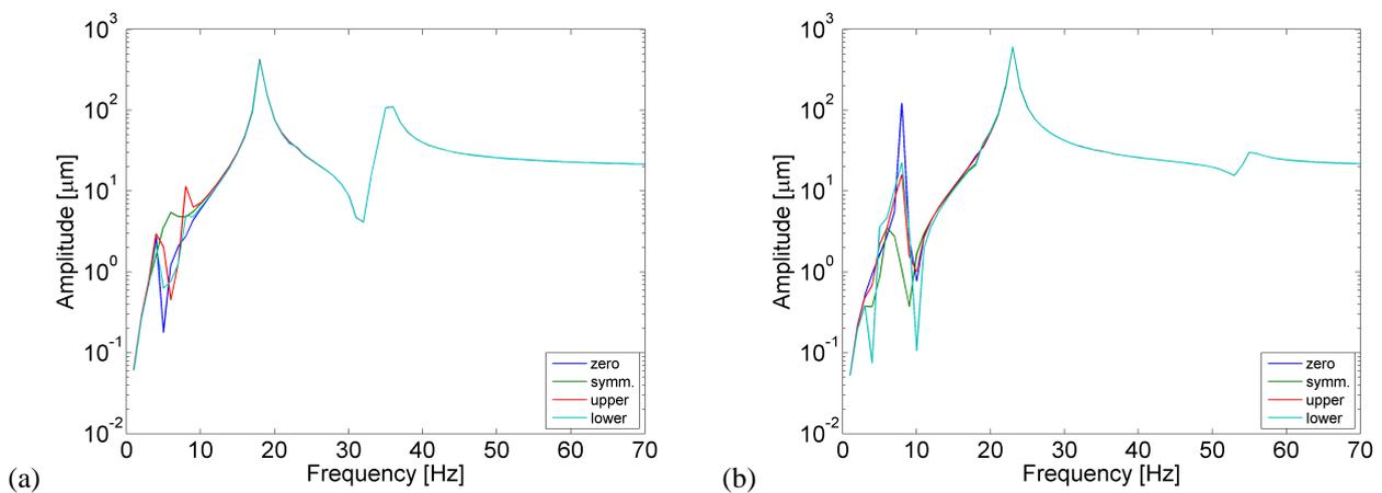
Fig. 10: Disk vibration amplitude (a – direction Y; b – direction Z) with modes 1 and 2 coupling.
