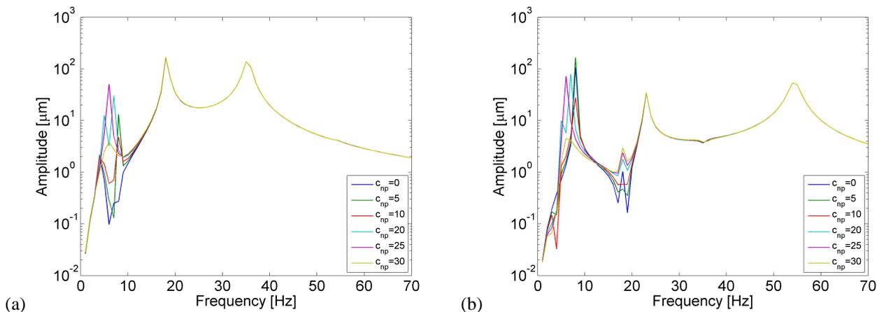
Fig. 5: Journal vibration amplitude (a – direction Y; b – direction Z) with modes 1 and 2 coupling.
