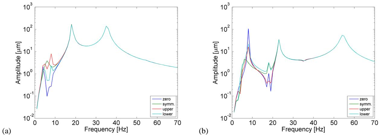
Fig. 11: Journal vibration amplitude (a – direction Y; b – direction Z) with coupling of modes 1 and 2.
