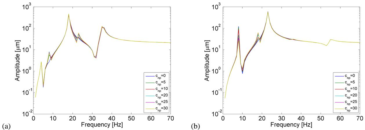
Fig. 7: Disk vibration amplitude (a – direction Y; b – direction Z) with modes 2 and 3 coupling.
