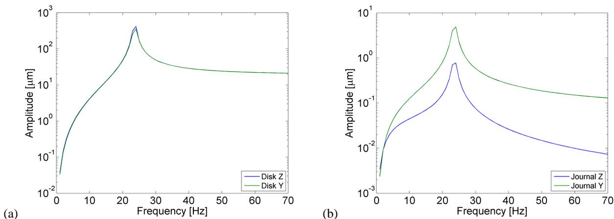
Fig. 3: Vibration amplitude of the rotor on a rigid foundation (a – disk; b – journal).
