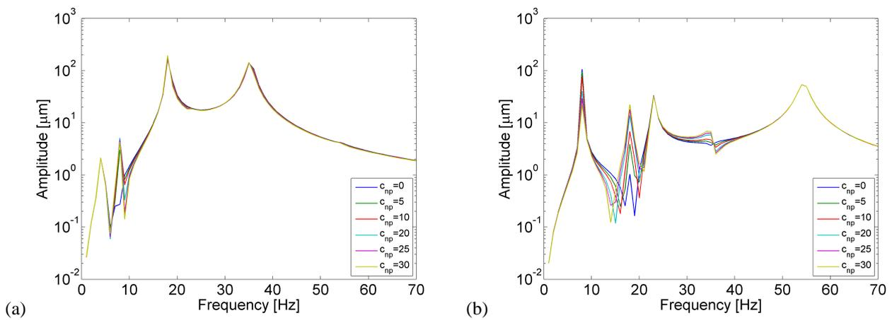
Fig. 8: Journal vibration amplitude (a – direction Y; b – direction Z) with modes 2 and 3 coupling.
