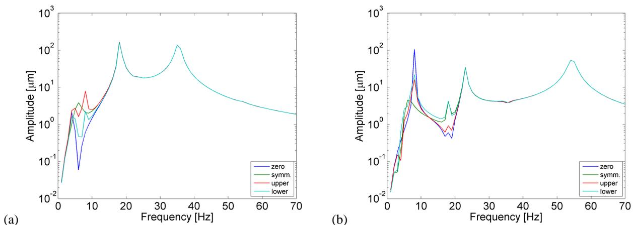
Fig. 12: Bearing case vibration amplitude (a – direction Y; b – direction Z) with modes 1 and 2 coupling.
