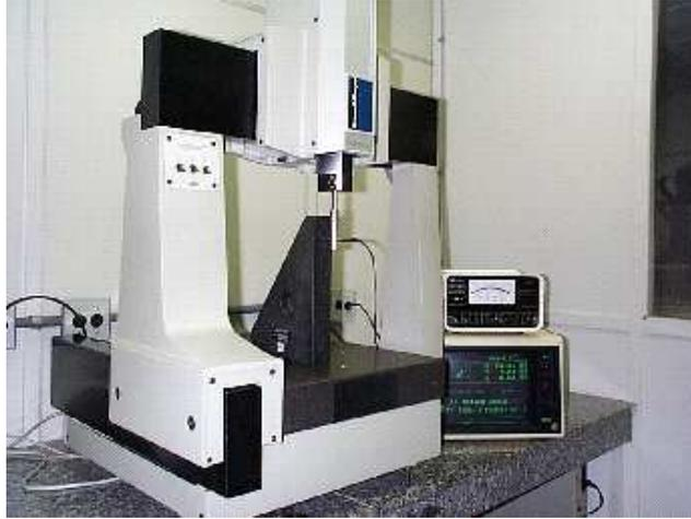
Figure 2. Moving Bridge type CMM.
