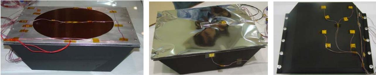
Figure 10 – Three views of VESPAR development model. Left: Bottom view of radiator without MLI (see circular heater attached to surface). Middle: Bottom view of radiator bottom (covered with MLI blanket). Right: Top view of second stage with TPs.
