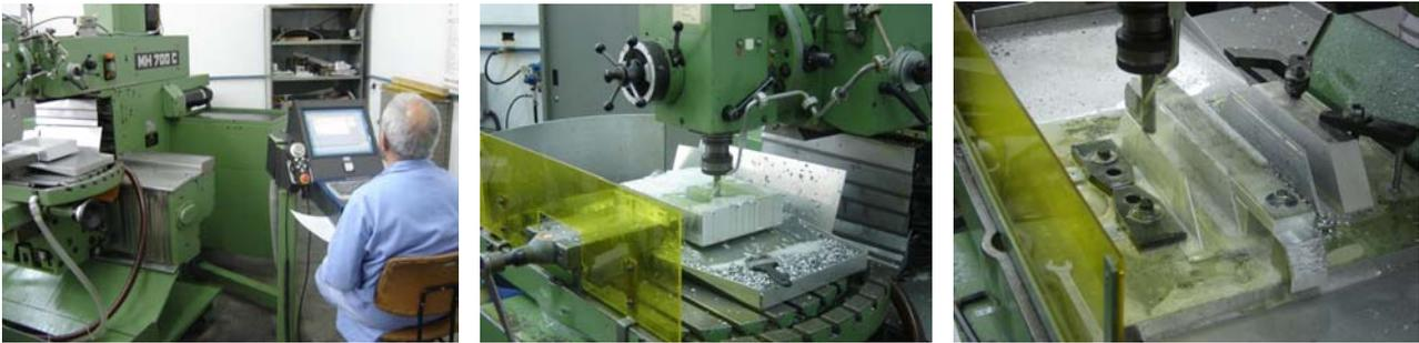
Figure 4 – Manufacturing of VESPAR stages.
