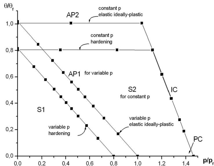
Figure 3. Hardening effect displayed in the sphere interaction diagram for  $\ell = 2.5$ . The numerical values are indicated by black squares. The lines are not analytical solutions but interpolation of the numerical values, plotted only to delimit the different domains. The elastic domain is not showed.
