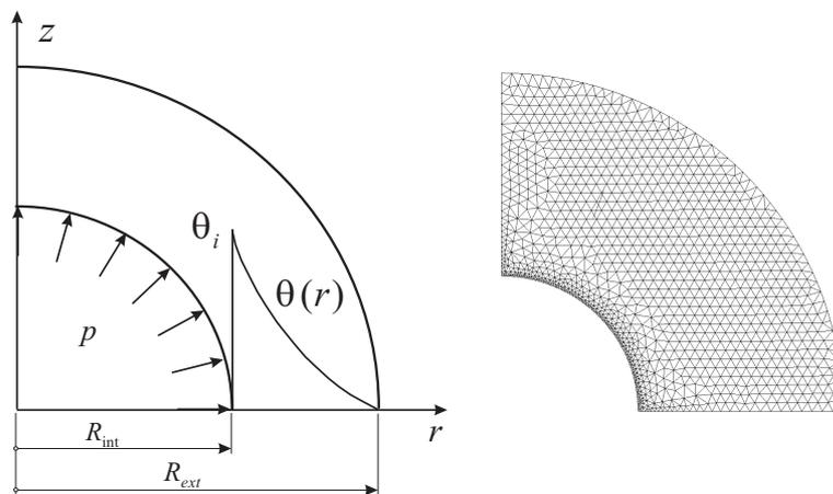
Figure 1. Temperature distribution through the sphere wall and the 2195 axisymmetric finite elements mesh.
