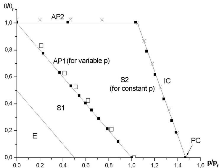
Figure 2. Comparison among numerical values obtained in this work (black squares) with those obtained by Yan (noted by X and by white squares) and with the analytical solutions (straight lines) for constant and variable  $p$ , for elastic ideally-plastic material and  $\ell = 2.5$ . The substantial reduction in the shakedown domain for variable  $p$  can be observed.
