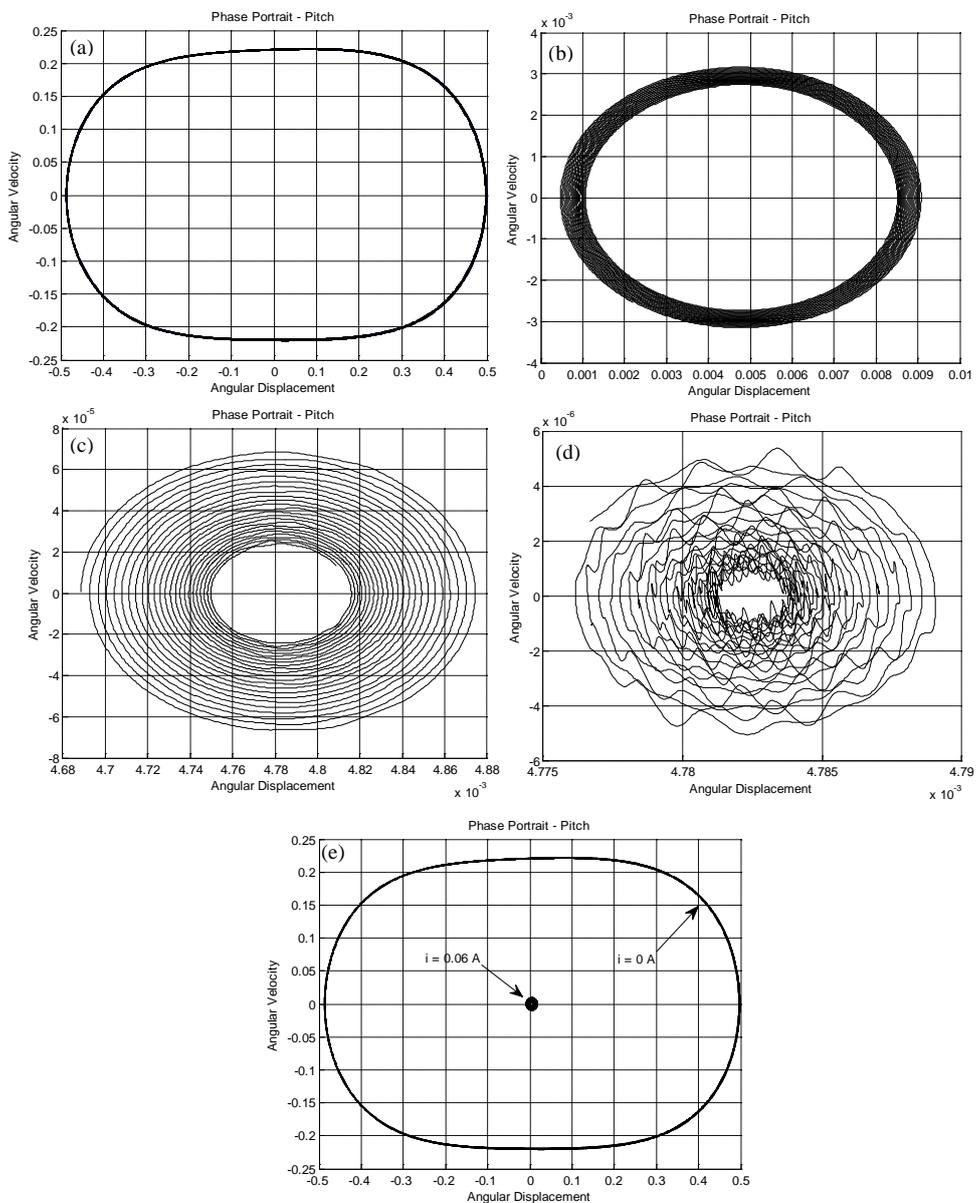
Figure 5. Evolution of Phase Portrait of Pitch degree of freedom,  $U = 20$  m/s, (a)  $i = 0A$ ; (b)  $i = 0.06A$ ; (c)  $i = 0.08A$ ; (d)  $i = 0.1A$ ; (e) LCO's Amplitude comparison.
