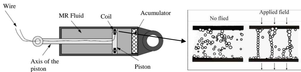
Figure 2 – Mechanical schema of MR damper and rheological behavior of MR fluid in the damper orifice.
