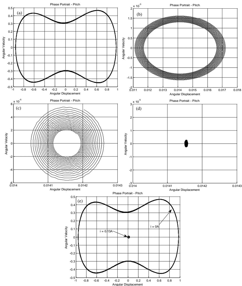
Figure 7. Evolution of Phase Portrait of Pitch degree of freedom,  $U = 25$  m/s, (a)  $i = 0A$ ; (b)  $i = 0.13A$ ; (c)  $i = 0.0.16A$ ; (d)  $i = 0.2A$ ; (e) LCO's Amplitude comparison.
