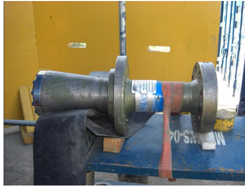
Figure 1. Assembled end fitting cut out from the pipe to analysis.
