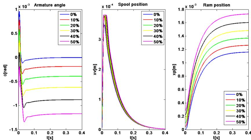
Figure 6. Closed loop response of the servovalve with nozzle orifice clogging. The nozzle orifice diameter is reduced in steps of 10% its nominal value.
