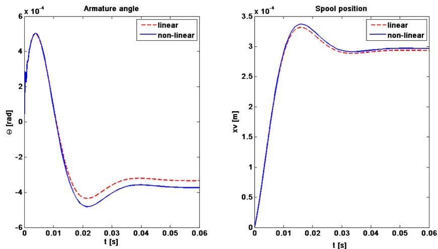
Figure 10. Open loop response of the servovalve with one nozzle orifice diameter reduced of 20% of its nominal value. Comparison of the non-linear model to the linear one.
