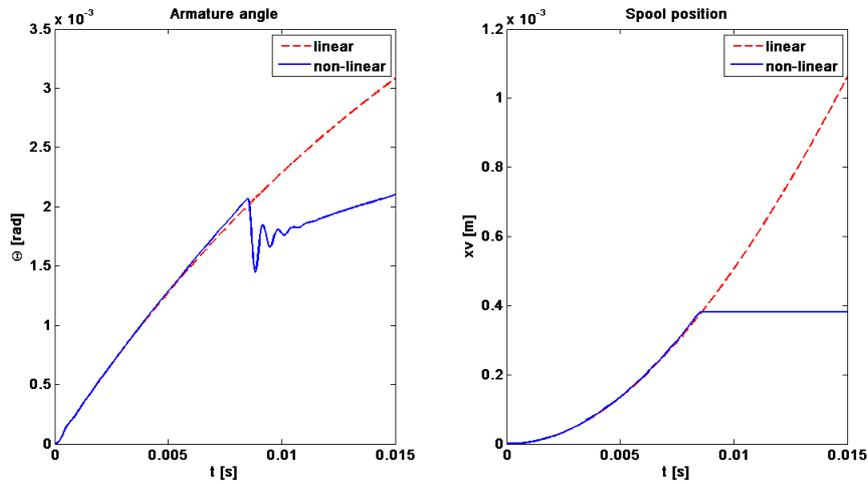
Figure 9. Open loop response of the servovalve with total loss of feedback spring. Comparison of the non-linear model to the linear one.
