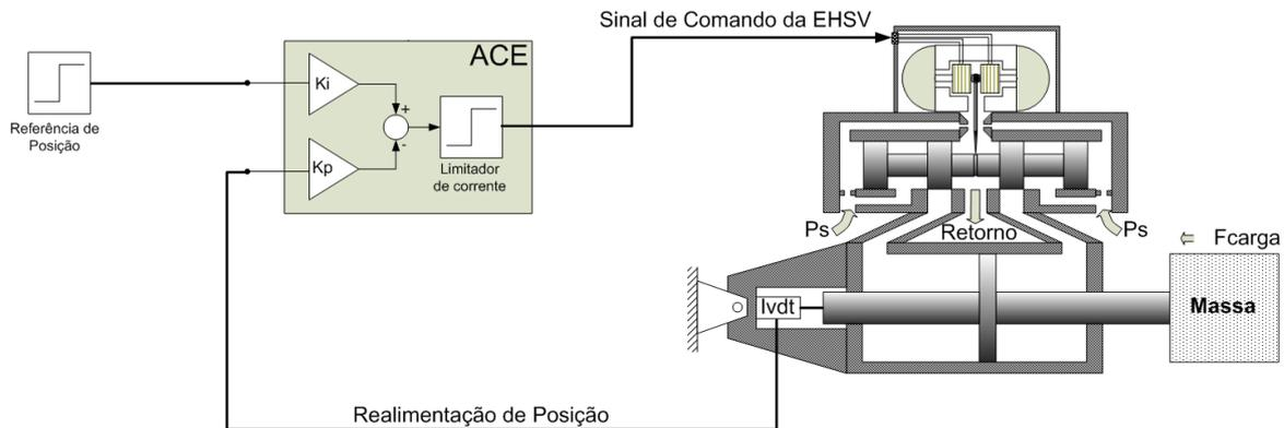
Figure 1. Diagram of the electrohydraulic servovalve under study together with a hydraulic actuator and a feedback controller.
