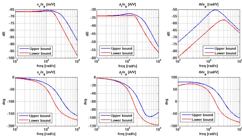
Figure 4. Frequency response operation envelope for the servovalve.
