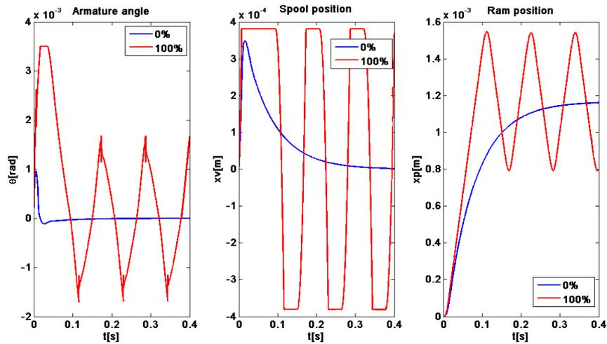
Figure 8. Closed loop response of actuator and servovalve with total loss of feedback spring.
