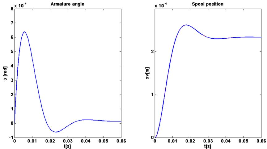
Figure 2. Open loop step response of the servovalve.
