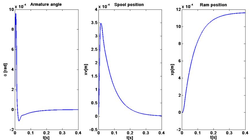
Figure 3. Closed loop step response of the servovalve and hydraulic actuator.
