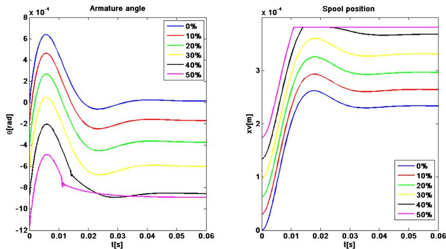
Figure 5. Open loop servovalve response with nozzle orifice clogging. The nozzle orifice diameter is reduced in steps of 10% its nominal value.
