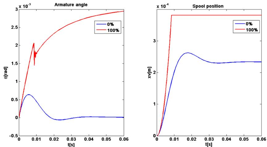
Figure 7. Open loop response of the servovalve with total loss of feedback spring.
