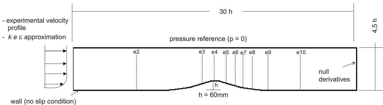
Figure 3. General outline of boundary conditions and geometrical characteristic.
