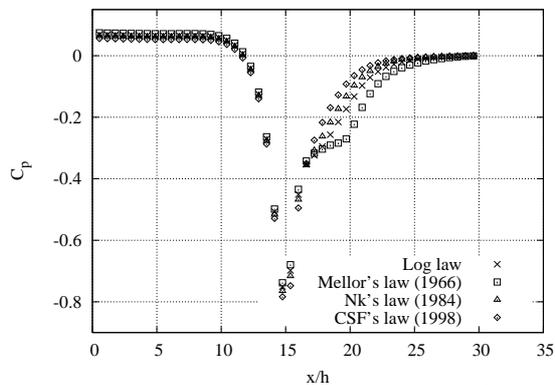
Figure 16. Longitudinal pressure gradient  $C_p$  using smooth laws.
