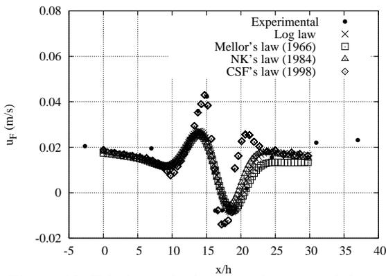
Figure 18. Friction velocity  $u_F$  using smooth laws.
