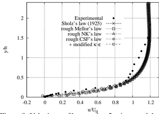
Figure 9. Velocity profile at station 5 using rough laws.
