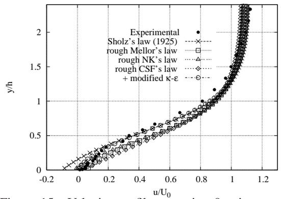
Figure 15. Velocity profile at station 9 using rough laws.
