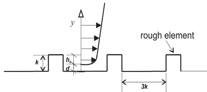
Figure 1. Roughness and the velocity profile origin.
