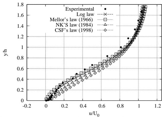
Figure 14. Velocity profile at station 9 using smooth laws.
