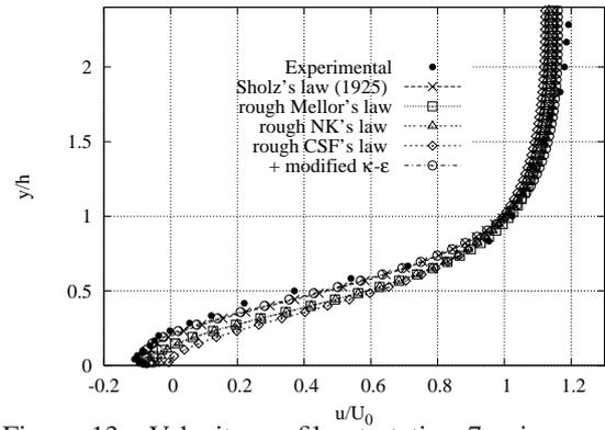
Figure 13. Velocity profile at station 7 using rough laws.
