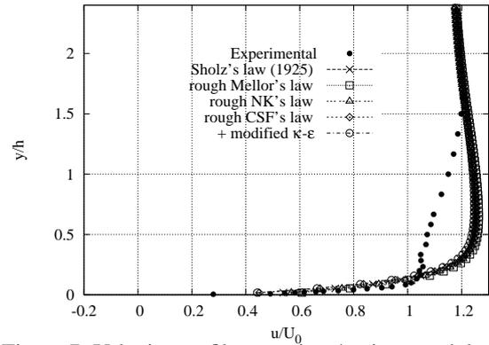
Figure 7. Velocity profile at station 4 using rough laws.
