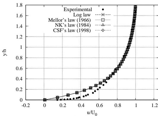
Figure 4. Velocity profile at station 2 using smooth laws.
