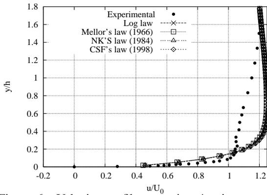
Figure 6. Velocity profile at station 4 using smooth laws.
