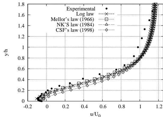
Figure 10. Velocity profile at station 6 using smooth laws.
