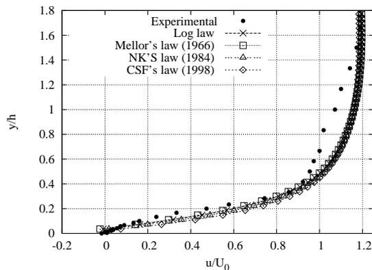
Figure 8. Velocity profile at station 5 using smooth laws.
