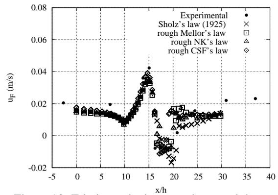
Figure 19. Friction velocity  $u_F$  using rough laws.
