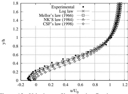
Figure 12. Velocity profile at station 7 using smooth laws.
