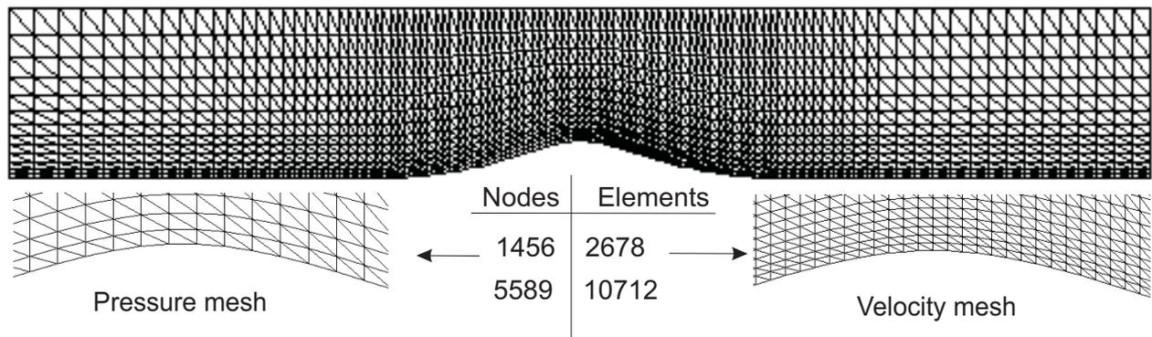
Figure 2. P1 and P1/ISO P2 meshes.
