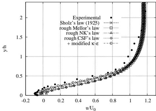
Figure 11. Velocity profile at station 6 using rough laws.
