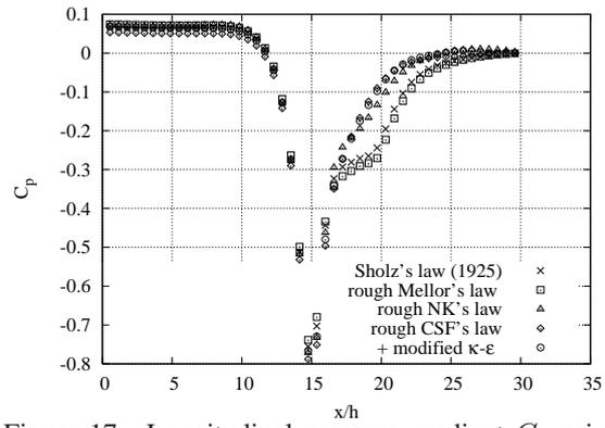
Figure 17. Longitudinal pressure gradient  $C_p$  using rough laws.
