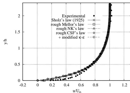
Figure 5. Velocity profile at station 2 using rough laws.
