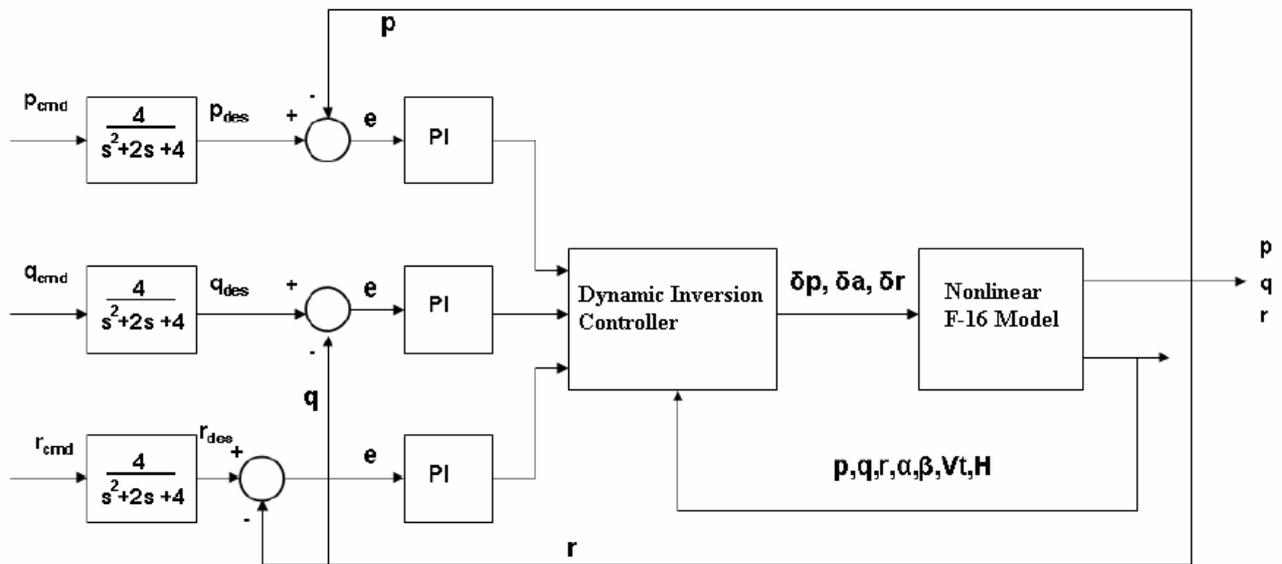
Figure 10. Develop Block Diagram with second order filter selected
