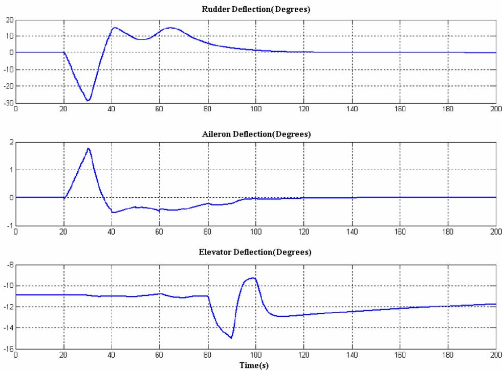
Figure 9. Surface movements to obtain the desired dynamic
