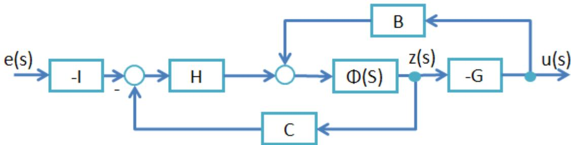
Figure 9 – Structure of the LQG/LTR controller based on the desired dynamics
