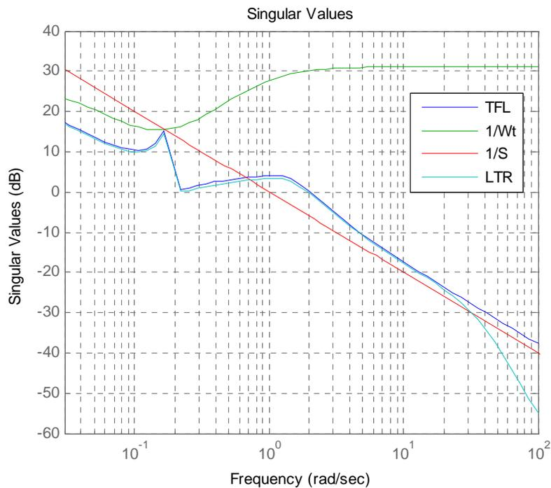
Figure 10 – Loop Transfer Recovery
