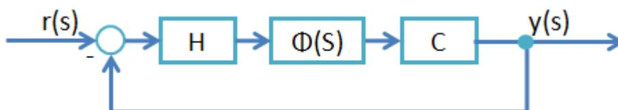
Figure 7 – Desired dynamic structure
