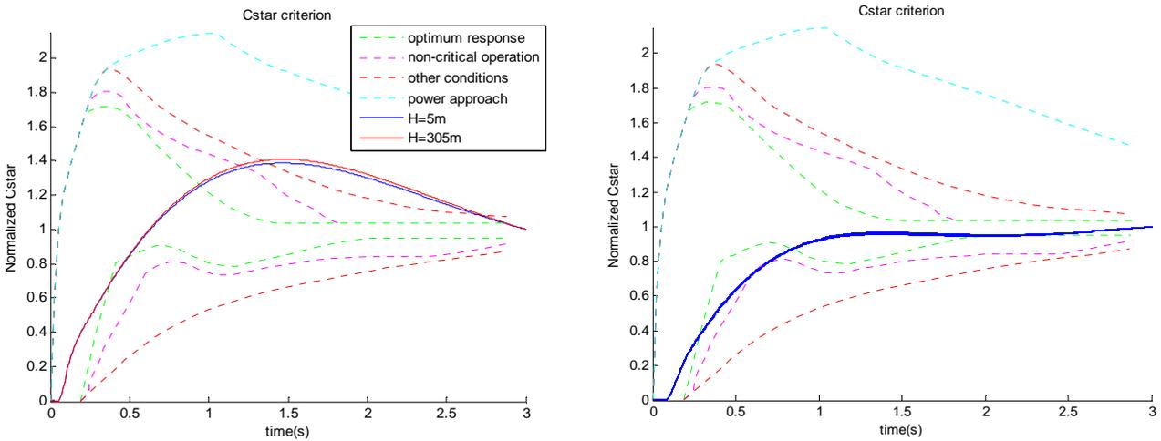
Figure 12 –  $C^*$  Criteria response (left – without the LQG/LTR controller / right – with the LQG/LTR controller)
