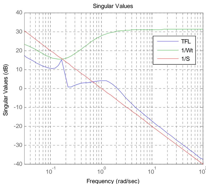
Figure 8 – Project of the Target Feedback Loop (TFL)
