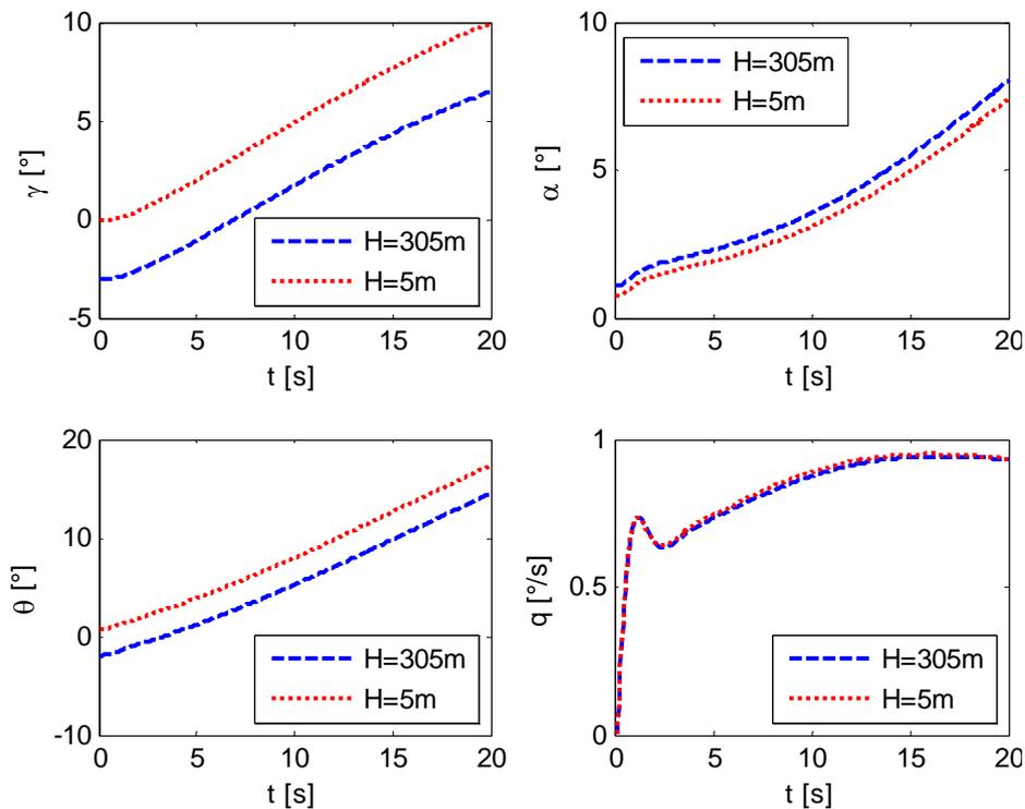
Figure 14 - Aircraft response with the LQG/LTR controller (b)
