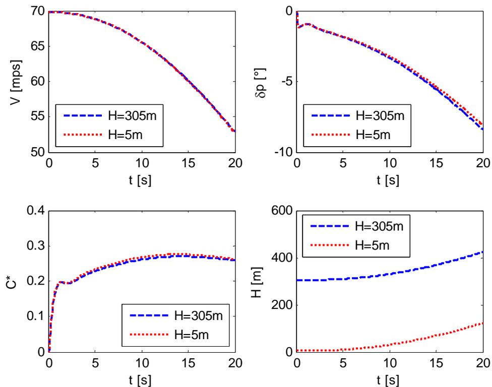
Figure 13 – Aircraft step response with the LQG/LTR controller (a)
