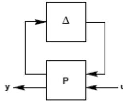
Figure 6. Upper Linear Fractional Transformation  $F_u(P, \Delta)$ .
