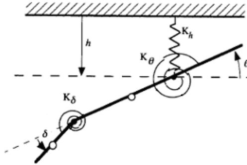
Figure 1. Aeroelastic *Typical Section* with Three Degrees of Freedom, Waszak (1998)
