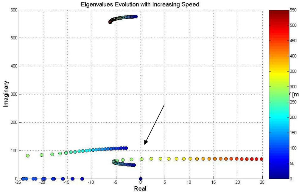
Figure 5. Nominal Plant Eigenvalues Evolution with Increasing Speed.
