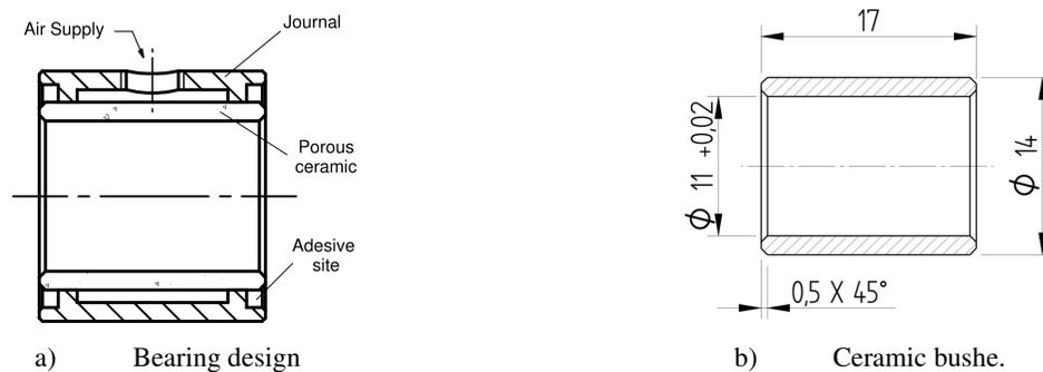
Figure 6 – Design of the aerostatic bearing with ceramic porous bushing.
