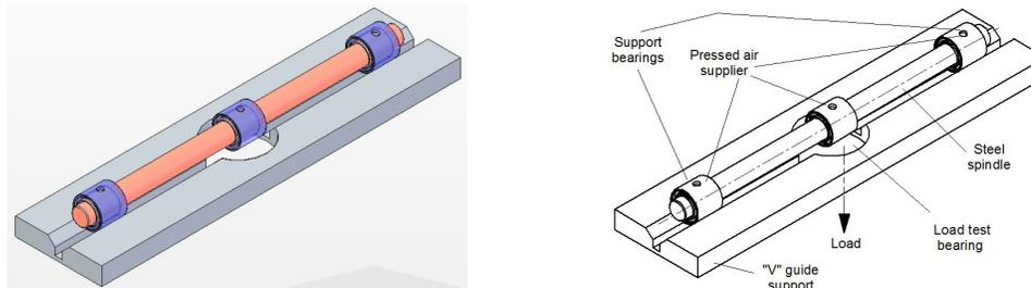
Figure 7 – Prototype obtained from TRIZ methodology.
