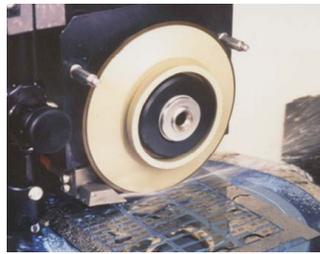
Figure 2 – Dicing Saw (GSI – Westwind, 2008)
