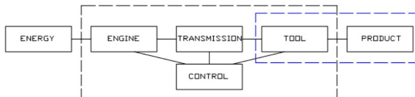
Figure 3 – Minimum structure for technical system.
