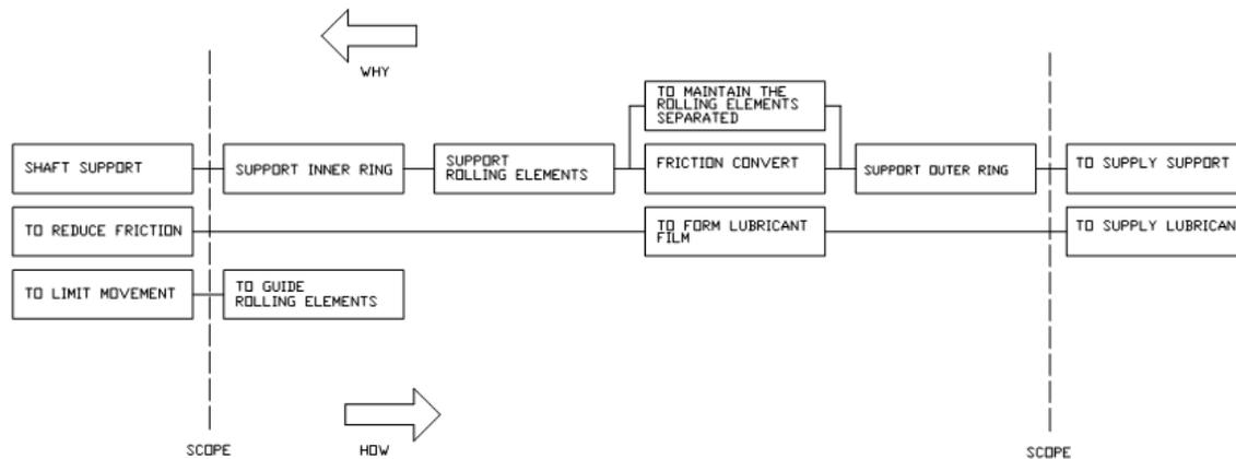
Figure 5 – Functional Tree of the “Bearing System”.
