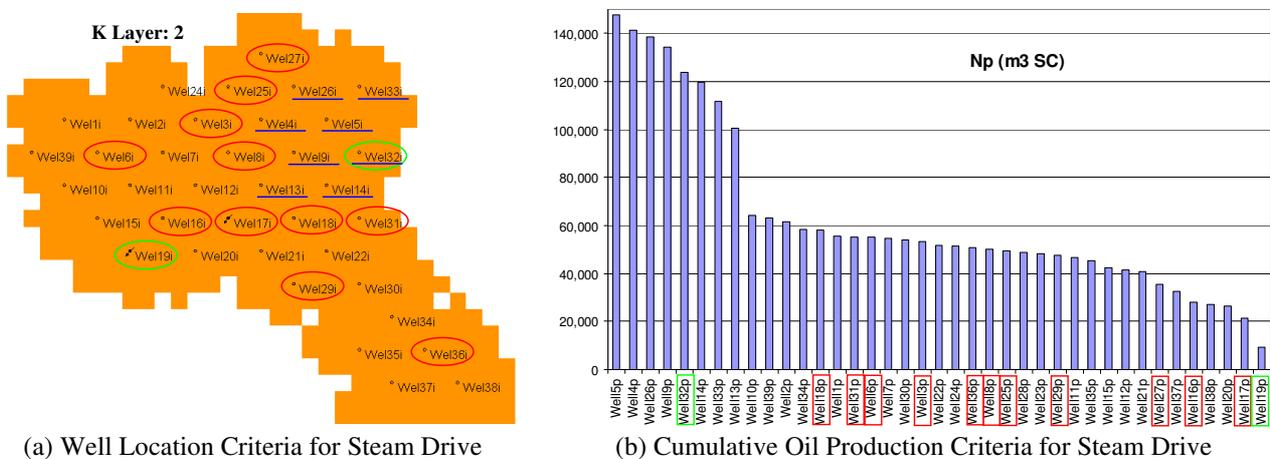
Figure 11. Methodology to Choose the Injector Wells for Steam Drive Phase.
