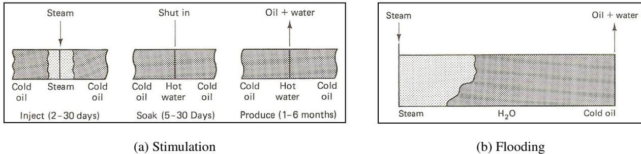
Figure 3. Steam Injection Processes (Lake, 1989).
