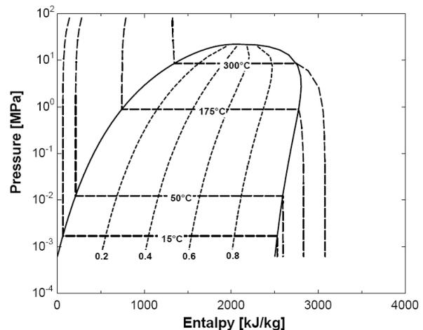
Figure 2. Water Pressure versus Enthalpy Diagram (Lake, 1989).
