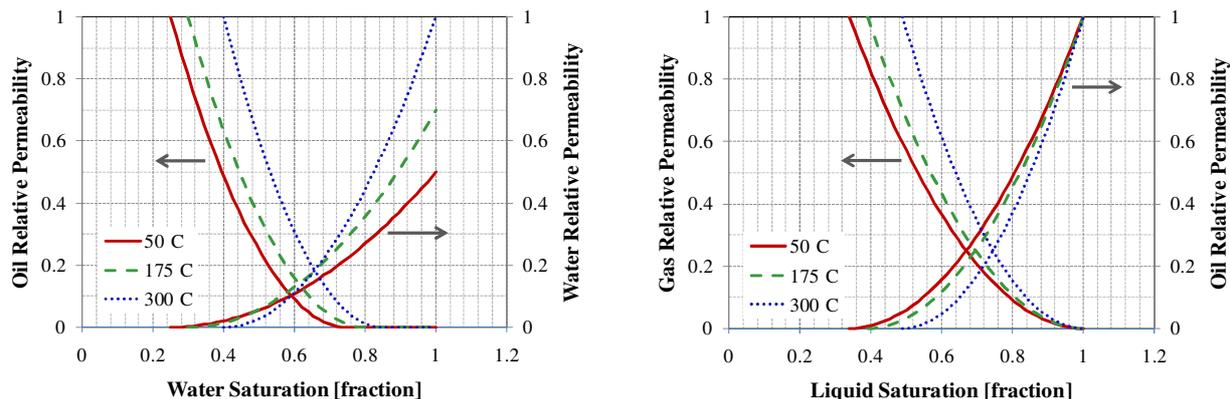
Figure 7. Relative Permeabilities (@50 C)
