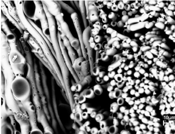
Figure 9. SEM quartz-phenolic after plasma jet exposure.
