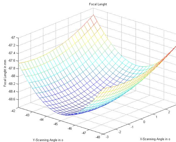
Figure 6. Focal length of the scanning system
