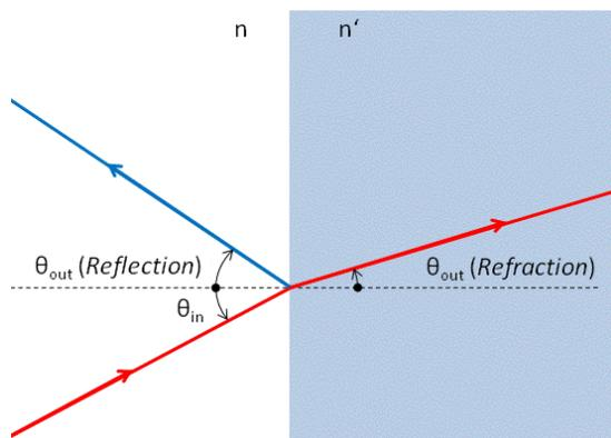
Figure 1. Reflection and refraction
