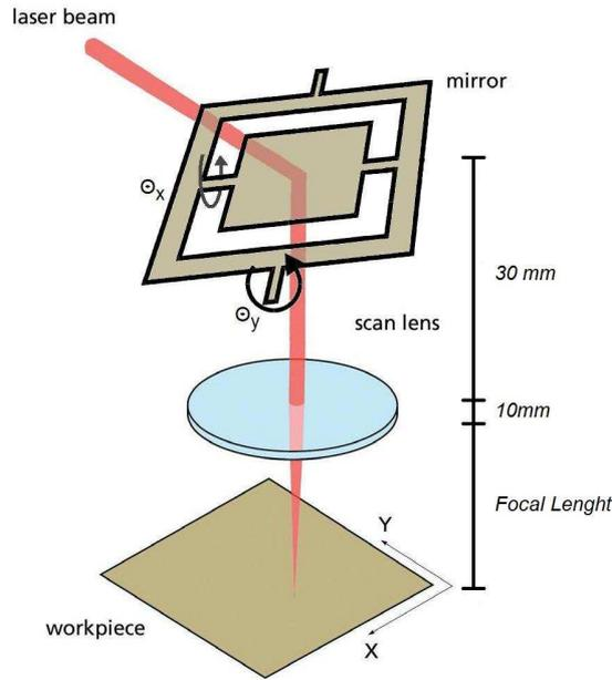
Figure 4. Simulation model of a 2D scanning system
