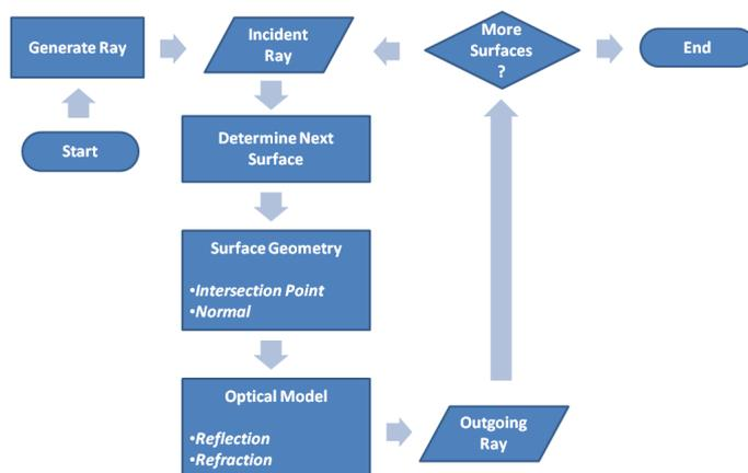
Figure 2. Ray-tracing flowchart
