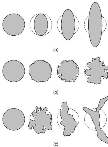
Figure 1. Three families of shape originated from a circle: (a) Ellipses with varied elongations; (b) rounded shapes with different irregularities; (c) combination of the previous cases (Adapted from Wojnar, 1999).
