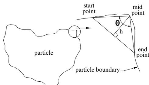
Figure 4. Method to calculate the spike parameter SP.
