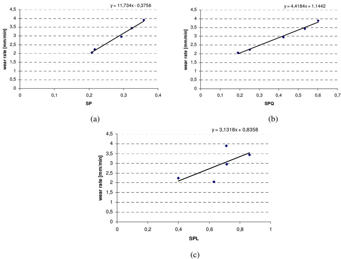
Figure 10. Plot of average wear rates vs. different spike parameters: (a) SP for different abrasive types, 20 particles measured for each abrasive type, (b) SPQ for different abrasive types, 20 particles measured for each abrasive type, (c) SPL for different abrasive types, only one particle measured for each abrasive type.
