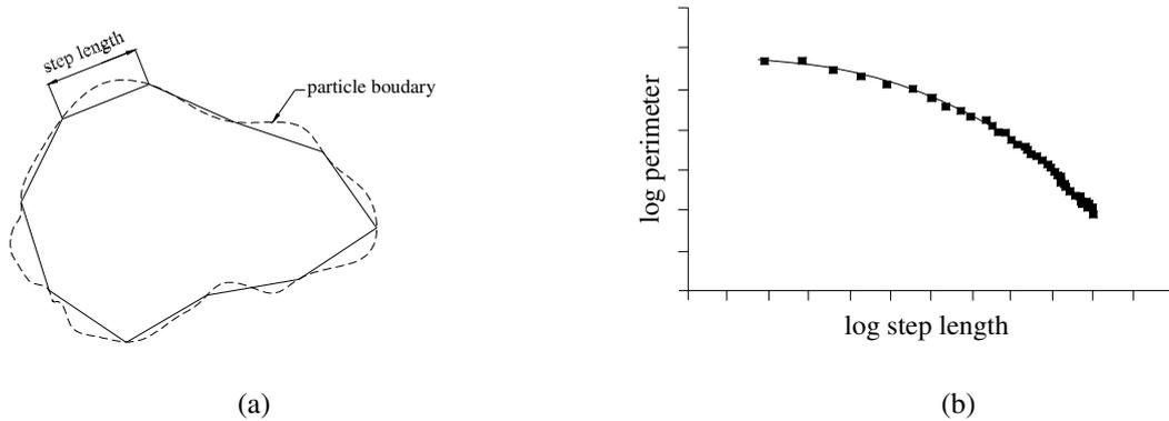
Figure 3. Richardson's curve for fractal dimension calculus.
