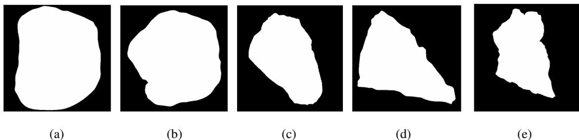
Figure 8. Abrasive grits: (a) silica sand, (b) garnet, (c) silicon carbide, (d) quartz, and (e) crushed sintered alumina. (Adapted from Hamblin and Stachowiak, 1996).
