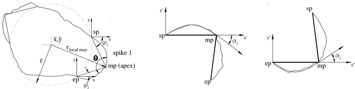
Figure 5. Method to the calculus of spike parameter SPQ.
