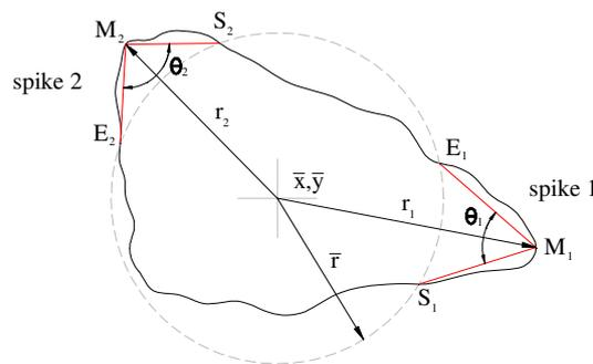
Figure 7. Methodology to calculate the modified spike parameter, SPL.
