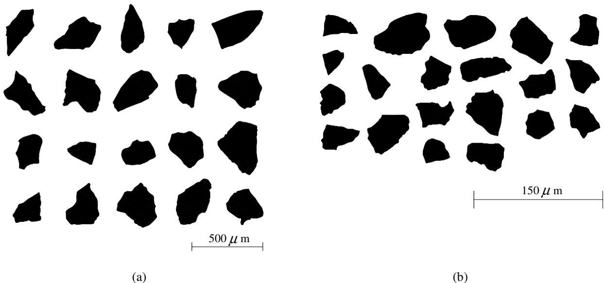
Figure 6. Binary images of glass particles: (a) 72  $\mu\text{m}$  and (b) 455  $\mu\text{m}$  average size.
