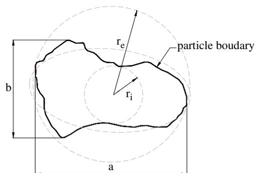
Figure 2. Geometry quantities required for the calculus of different shape factors.
