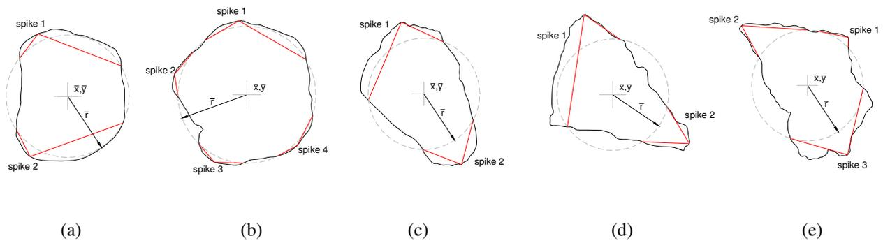
Figure 9. Details of detected spikes for each mineral: (a) silica sand, (b) garnet, (c) silicon carbide, (d) quartz, and (e) crushed sintered alumina.
