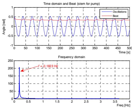
Figure 7. Oscillations of stem with response in time domain and frequency domain.
