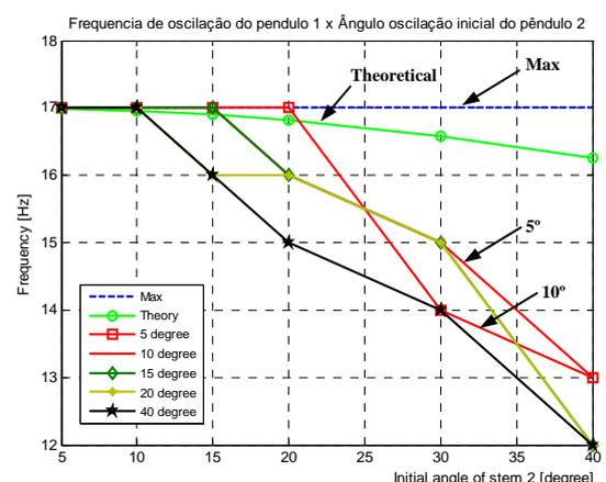
Figure 19. Frequency variation for stem 1 versus initial angle for stem 2.
