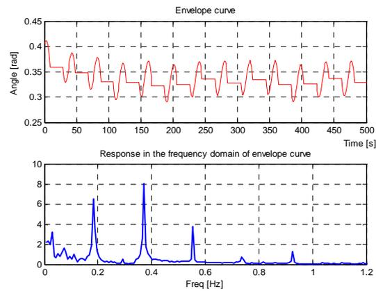
Figure 8. Envelope Curve of sinusoidal term and response in frequency.
