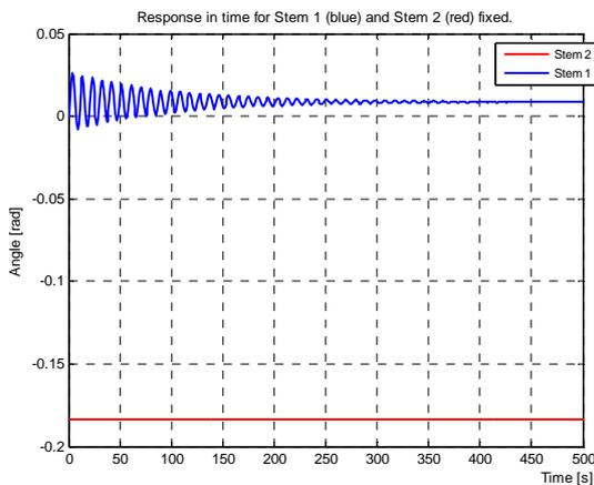
Figure 14. Response in time domain for stem 1 with stem 2 fixed.
