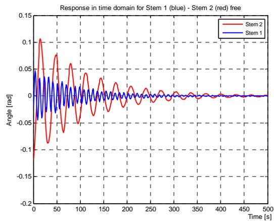
Figure 15. Response in time domain for stem 1 and stem 2 free,
