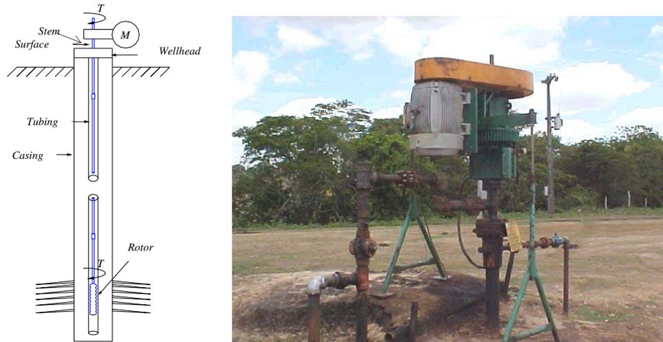
Figure 1. Configuration of oil well equipped with typical BCP installation (electric motor and headstock).
