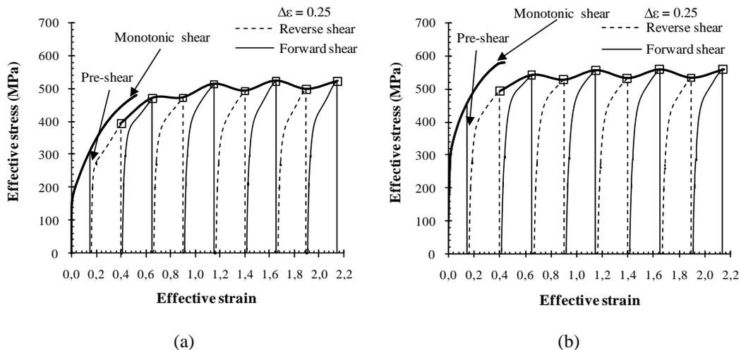
Figure 7. Effective stress versus accumulated effective strain curves after cyclic test with  $\Delta\varepsilon = 0.25$ : (a) annealed brass and (b) work hardened brass.
