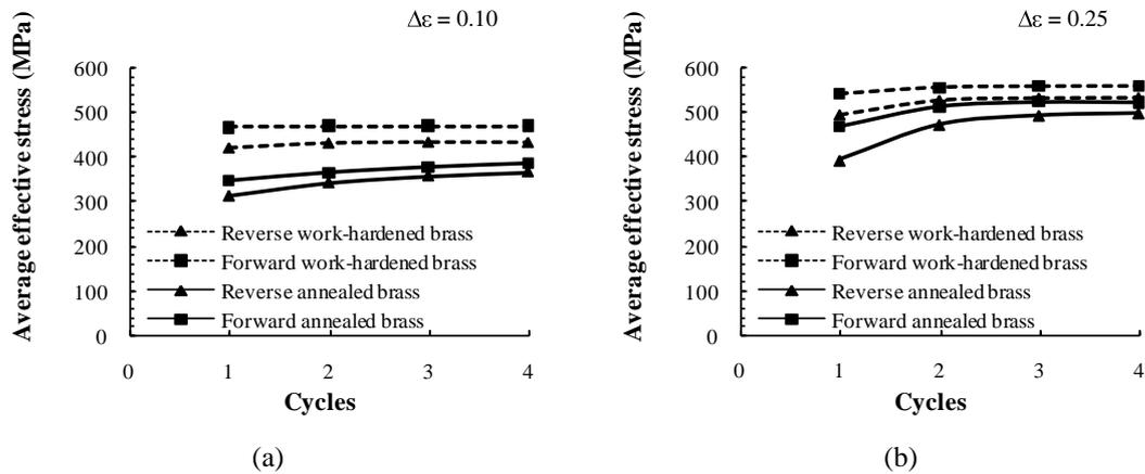
Figure 8. Average effective stress versus number of cycles for plastic strain amplitude of: (a) 0.10 and (b) 0.25.
