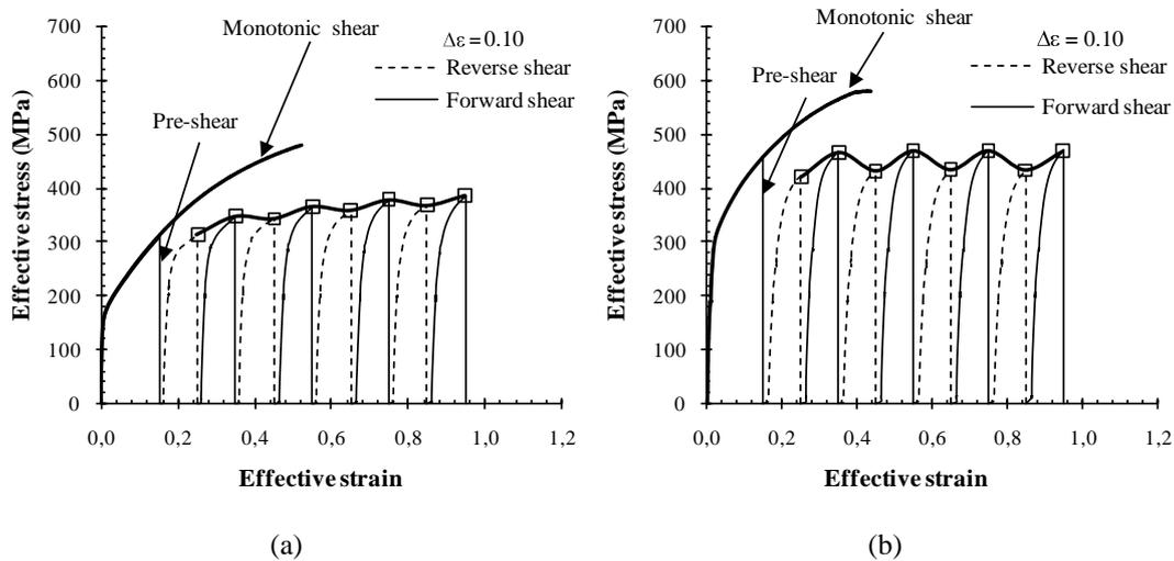
Figure 5. Effective stress versus accumulated effective strain curves after cyclic test with  $\Delta\varepsilon = 0.10$ : (a) annealed brass and (b) work hardened brass.
