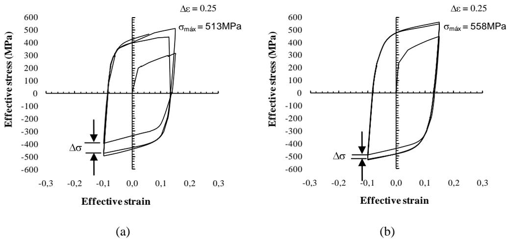
Figure 6. Effective stress versus accumulated effective strain curves after cyclic test with  $\Delta\varepsilon = 0.25$ : (a) annealed brass and (b) work hardened brass.
