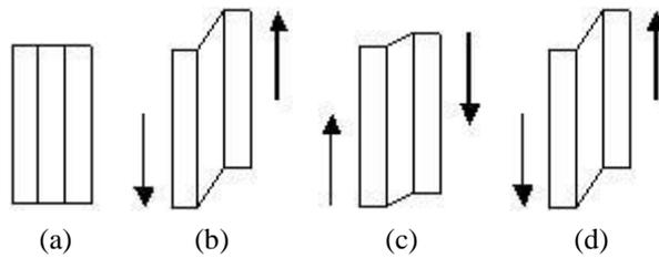
Figure 2. Specimen shearing during the cyclic test with  $\Delta\varepsilon = 0.10$ : (a) non-deformed, (b) prestraining up to 0.15 under forward shear, (c) reverse shear up to 0.10 and (d) last step of cyclic route: forward shear up to 0.10.
