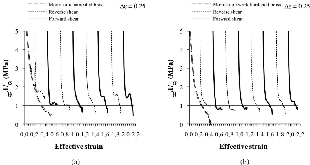
Figure 9. Normalized work hardening rate versus effective strain for cyclic strain amplitude of  $\Delta\varepsilon = 0.25$ : a) annealed brass and (b) work hardened brass.
