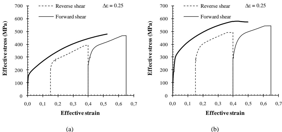
Figure 10. Effective stress versus effective strain for first cycle with  $\Delta\varepsilon = 0.25$ : a) annealed brass and b) work hardened brass.
