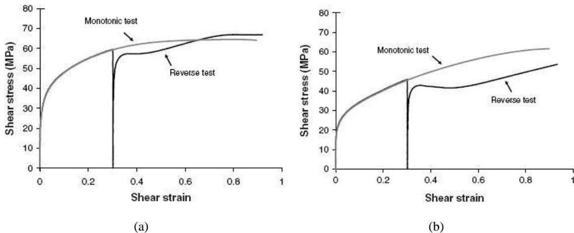
Figure 1. Shear stress versus shear strain curves for AA1050-O aluminum alloy under Bauschinger test: a) reverse shear along the rolling direction (0°RD) and b) reverse shear at 45° to the rolling direction (45°RD), Rauch *et al.* (2007).
