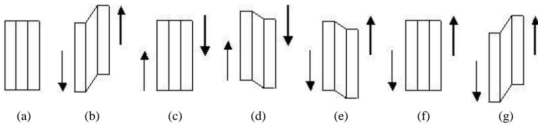
Figure 3. Models of the shear specimen during the cyclic test with  $\Delta\varepsilon = 0.25$ : (a) non-deformed, (b) prestraining up to 0.15 under forward shear, (c) reverse shear of 0.15 (d) additional reverse shear of 0.10 (e) start of forward shear (f) forward shear up to 0.15 and (g) additional forward shear up to 0.25.
