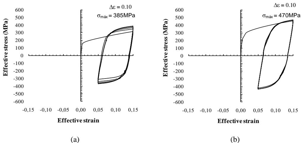
Figure 4. Effective stress versus effective strain curves obtained after the cyclic test with  $\Delta\varepsilon = 0.10$ : (a) annealed brass and (b) work hardened brass.
