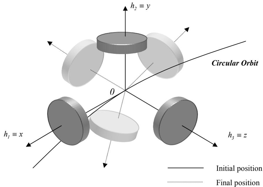
Figure 1 – Change on the angular positions of a satellite with three internal wheels
