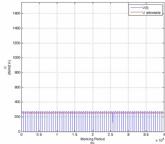
Figure 7. U trend through 5 years for the “TGA3” exchanger.
