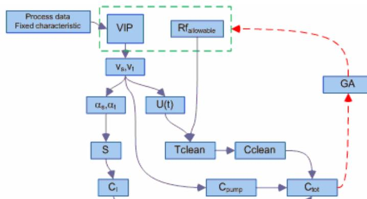
Figure 3. Flow chart of optimization procedure using GA and considering maintenance
