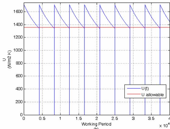
Figure 4. U trend through 5 years for the “Joint Optimization” exchanger.
