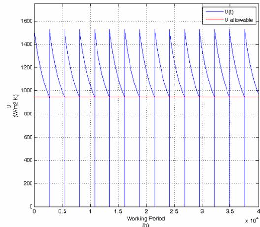
Figure 5. U trend through 5 years for the “TGA1” exchanger.
