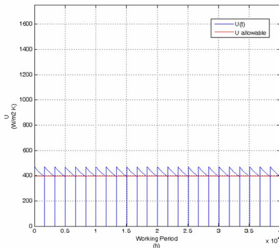
Figure 6. U trend through 5 years for the “TGA2” exchanger.
