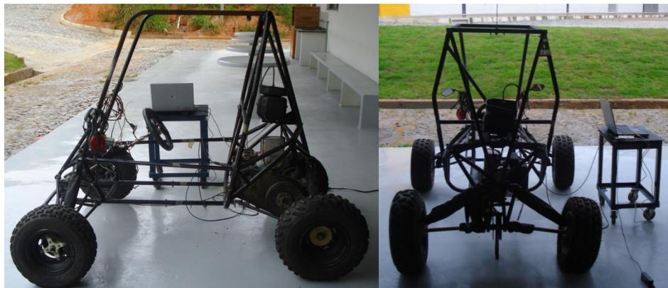
Figure 3. Data acquisition to perform the ODS analysis.
