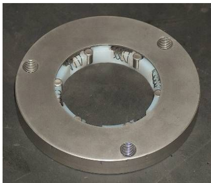
Figure 6. Starter OWC for Honda CG 125cc motorcycle (Courtesy: ZEN S.A.)
