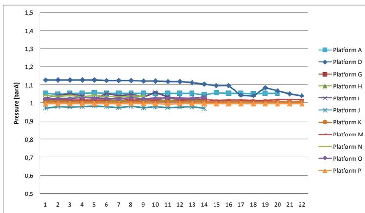
Figure 2 – Readings of gas pressure in flare tube [barA]
