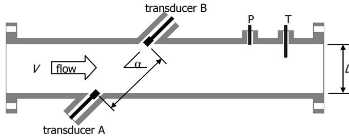
Figure 1 – Ultrasonic meter scheme and basic dimensions
