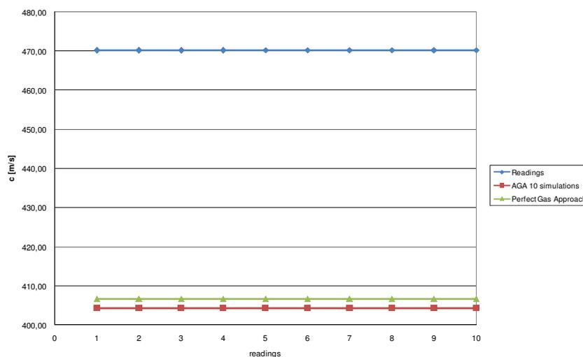
Figure 10 – Plots of operational readings of SOS measured at platform A compared with AGA-10 simulations and perfect gas approach.
