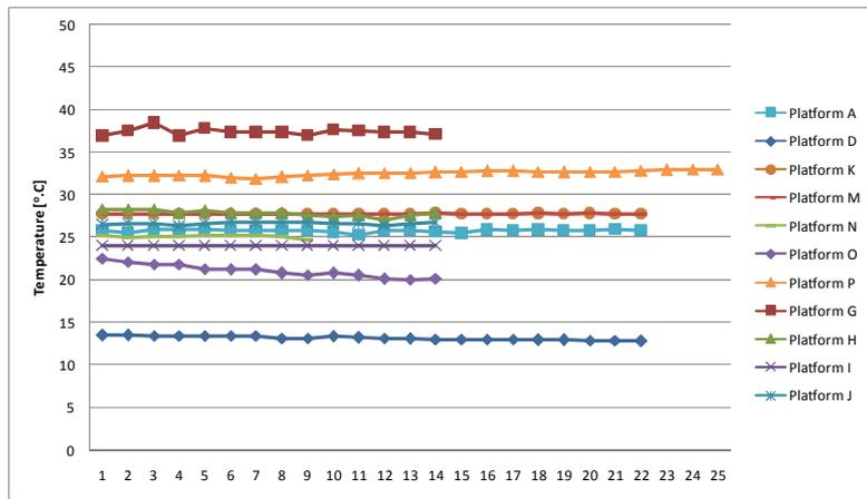
Figure 3 – Readings of gas temperature in flare tube [°C]
