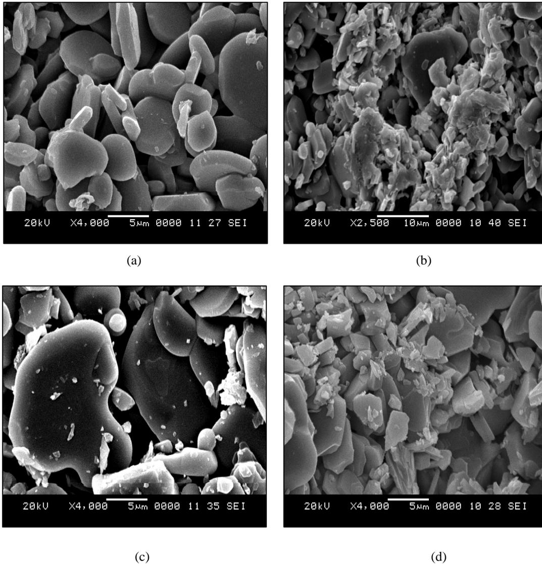
Fig. 5 SEM micrographs of  $\text{Al}_2\text{O}_3\text{-TiO}_2$  ceramic composites with 1 wt% of  $\text{CeO}_2$  additives, (a) 5% wt  $\text{TiO}_2$ , (a)5% wt  $\text{TiO}_2$ , (b) 10% wt  $\text{TiO}_2$ , (c) 15% wt  $\text{TiO}_2$ , (d) 20% wt  $\text{TiO}_2$ ,
