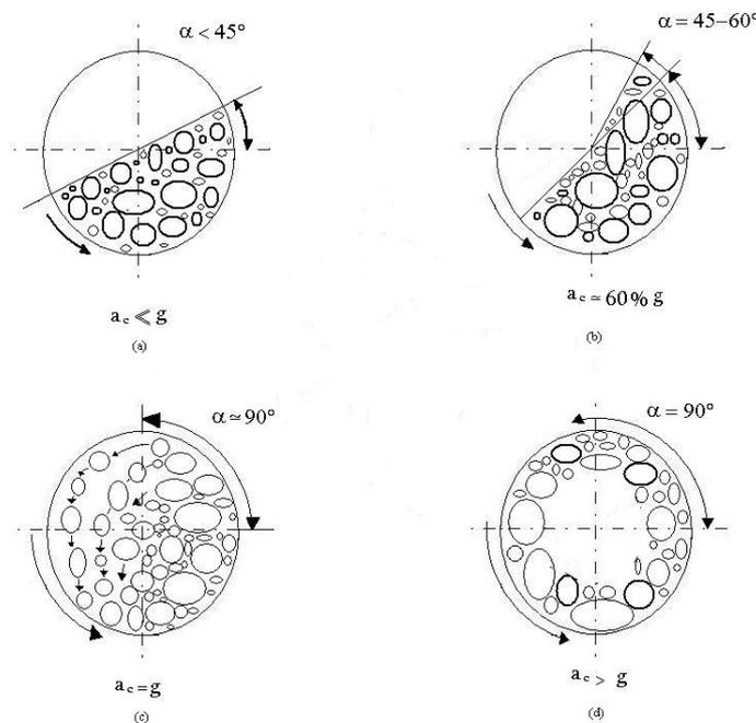
Fig.1. Schematic illustration of interior of a ball mill for four different values of the centrifugal accelerations ( $a_c$ ),  $\beta$  - angle of cascade
