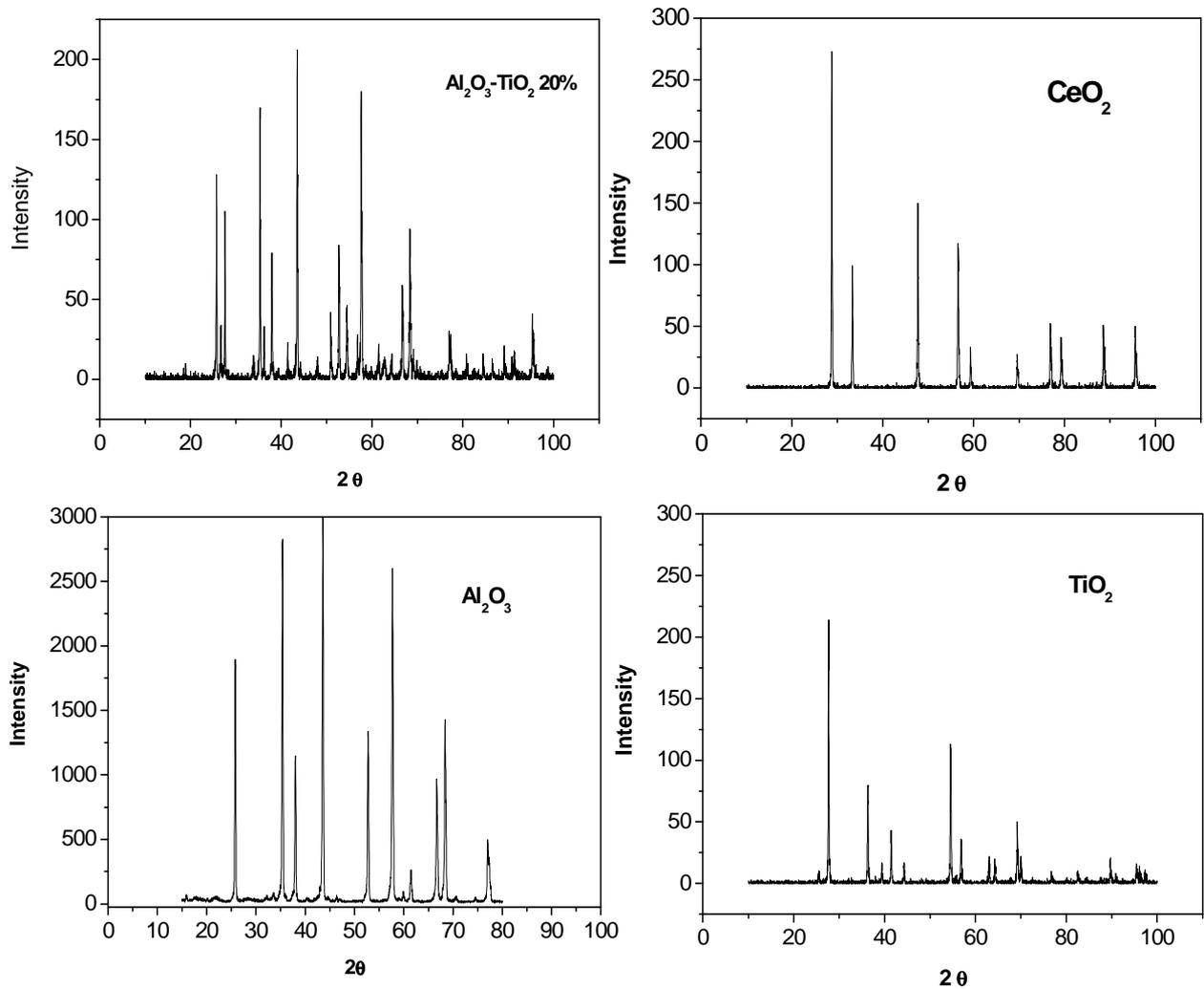
Fig. 2. X-ray Diffraction spectrum of  $\text{Al}_2\text{O}_3$ - $\text{TiO}_2$  ceramic composites with 1 wt% of  $\text{CeO}_2$  additives along with the XRD spectra of constituent ceramics  $\text{TiO}_2$ ,  $\text{Al}_2\text{O}_3$ ,  $\text{CeO}_2$  ceramics used for the fabrication of composites for easy comparison
