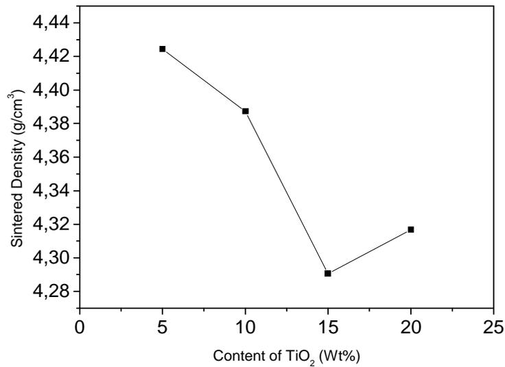
Fig. 3 Sintered density of Al<sub>2</sub>O<sub>3</sub>-TiO<sub>2</sub> ceramic composites with 1 wt% of CeO<sub>2</sub> additives
