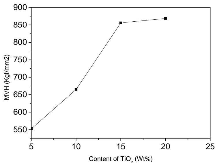
Fig. 4 Vicker's microhardness of Al<sub>2</sub>O<sub>3</sub>-TiO<sub>2</sub> ceramic composites with 1 wt% of CeO<sub>2</sub> additives
