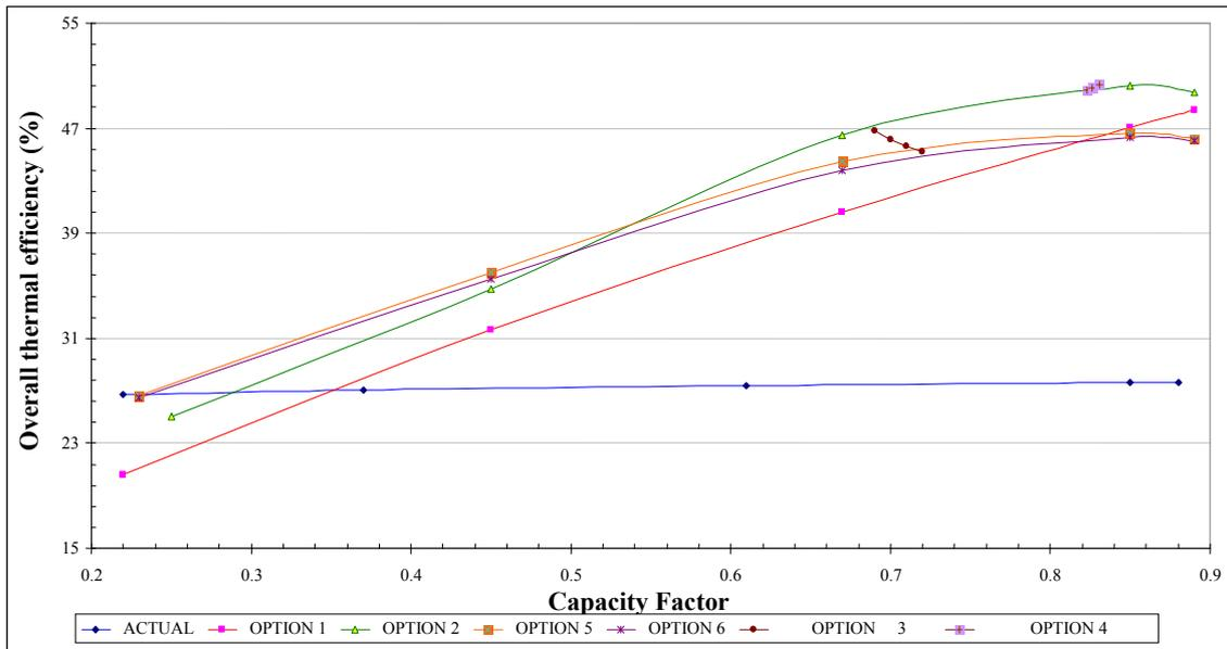
Figure 2. Overall thermal efficiency of the U2 power plant (currently and repowering)
