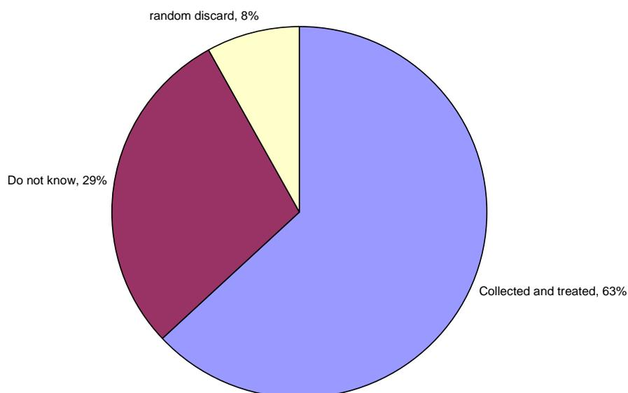
Figure 6. Destiny of cutting fluids
