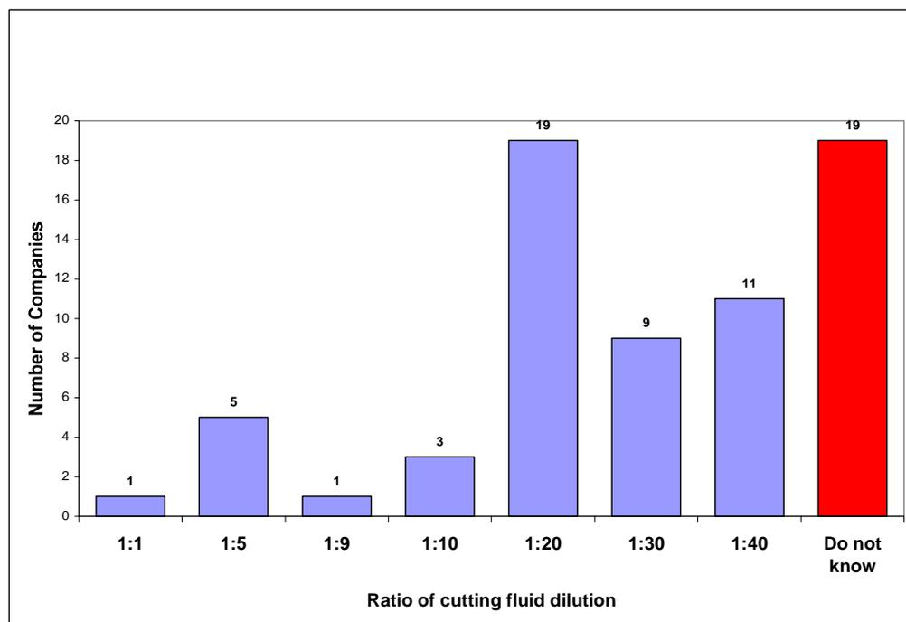
Figure 3. Ratios of dilution of cutting fluids
