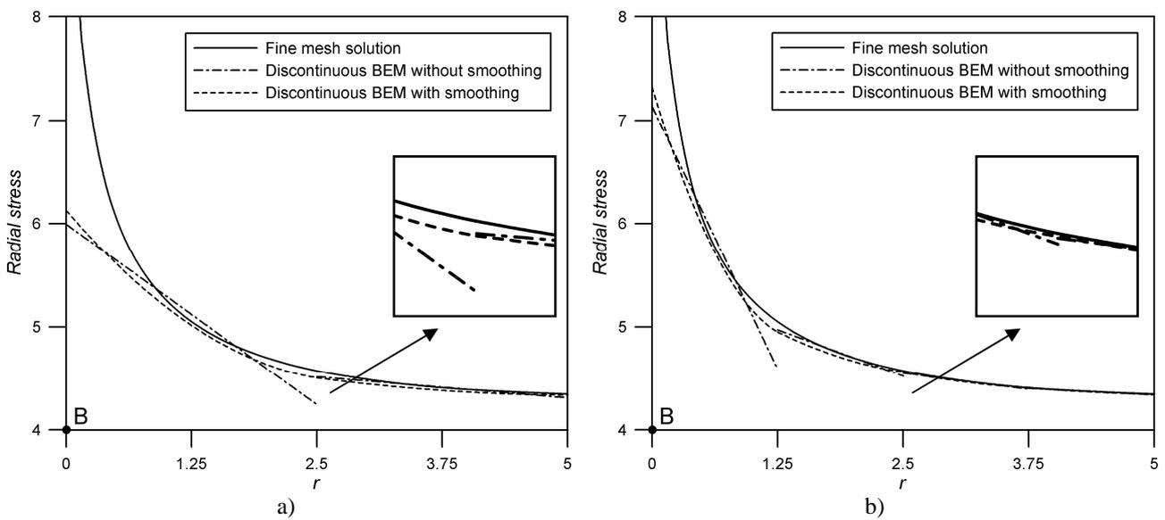
Figure 11. Radial stress recovery along edge BC. Quadratic elements: (a) mesh 1, (b) mesh 2.
