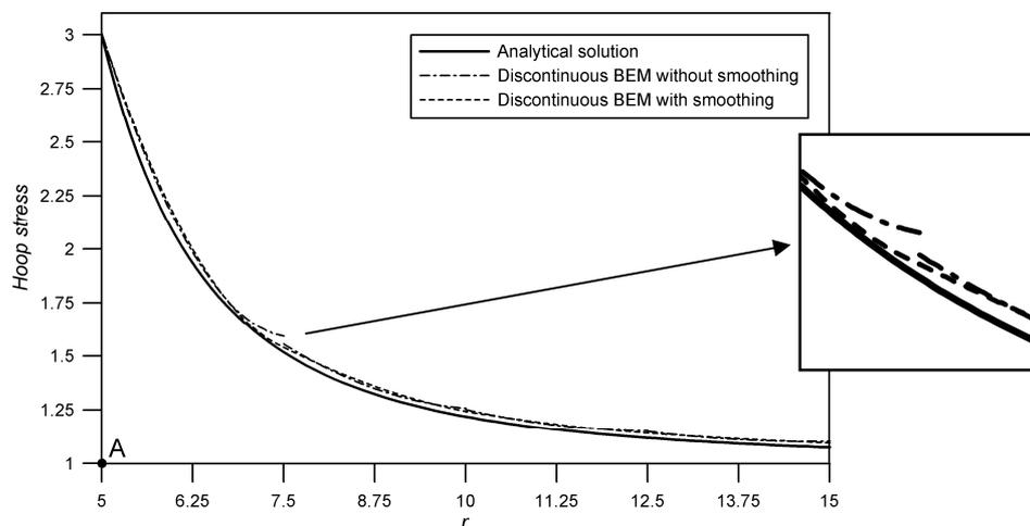
Figure 6. Hoop stress smoothing results for squared plate with central hole. Quadratic elements – mesh 1.
