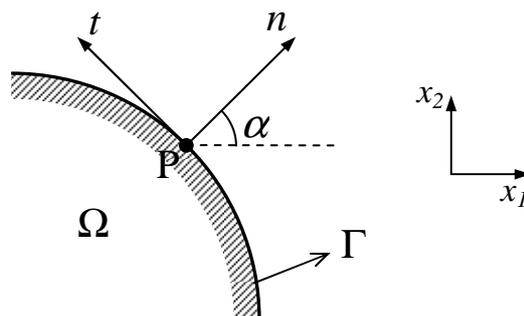
Figure 3. Coordinate system over the boundary.
