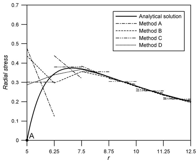
Figure 8. Radial stress recovery along edge AB. Linear elements – mesh 2.
