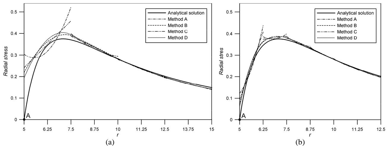
Figure 9. Radial stress recovery. Quadratic elements: (a) mesh 1, (b) mesh 2.
