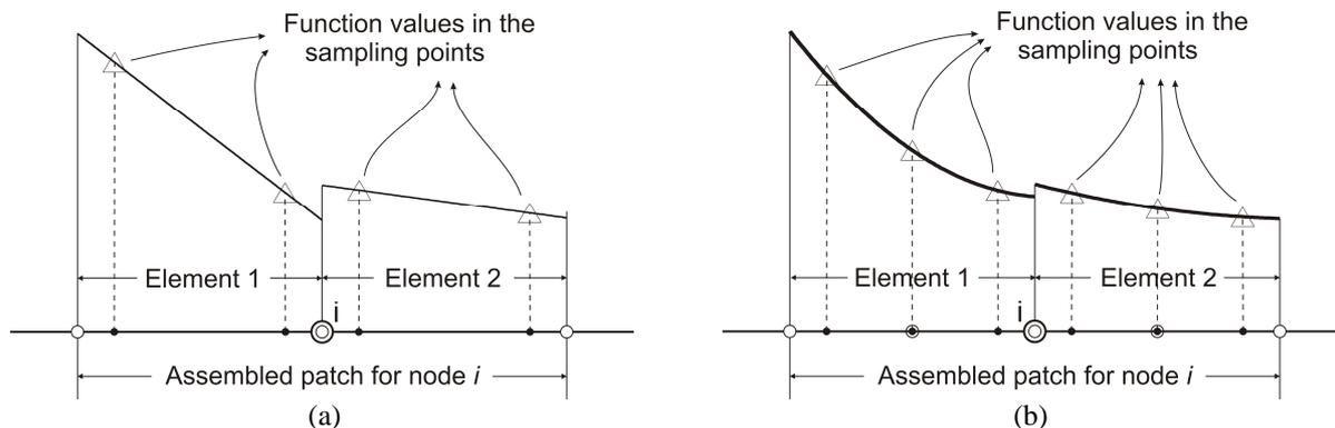
Figure 1. Discontinuous boundary element patches. (a) linear elements; (b) quadratic elements.
