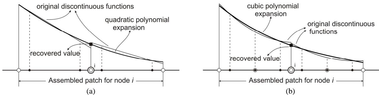
Figure 2. Variable recovery on a shared node. (a) Linear elements; (b) Quadratic elements.
