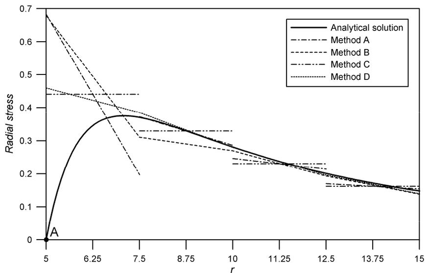
Figure 7. Radial stress recovery along edge AB. Linear elements – mesh 1.
