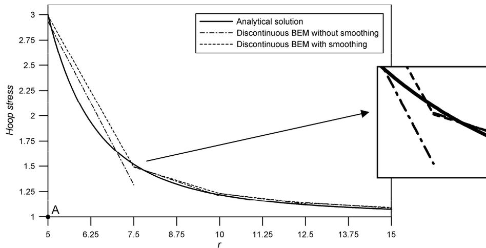
Figure 5. Hoop stress smoothing results for squared plate with central hole. Linear elements – mesh 1.
