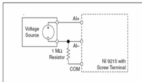
Figure 1. Connection of a floating differential voltage signal to the NI 9215 with Screw terminal
