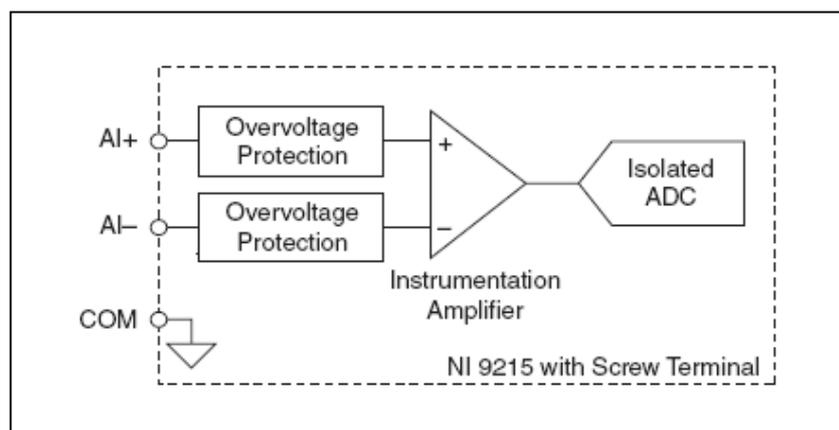
Figure 2. Input circuit for one channel on the NI 9215 with Screw terminal
