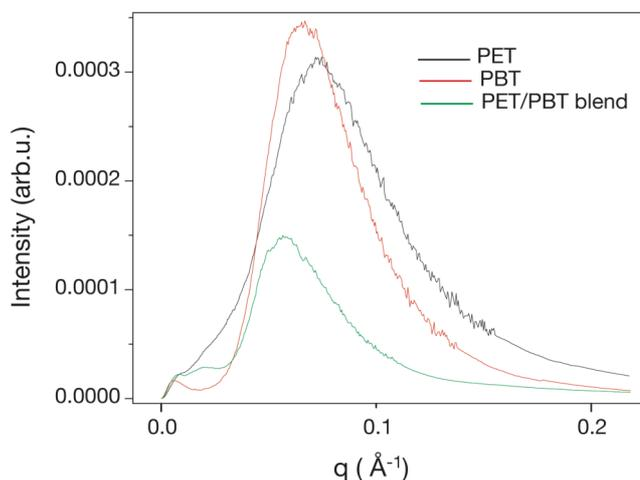
Figure 5. One-dimensional SAXS curves for the neat polymers and PET/PBT blend.
