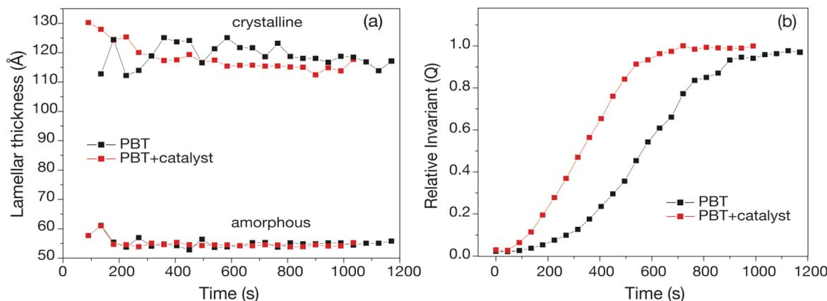
Figure 3. Time evolution of the crystalline parameters of the PBT with and without catalyst during the crystallization at 210 °C.
