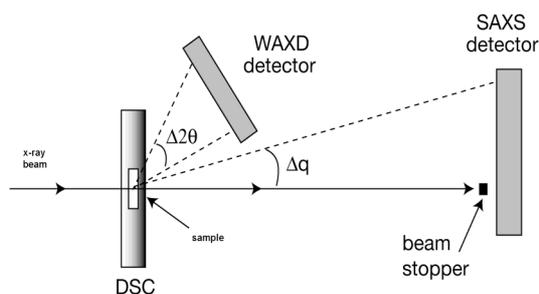
Figure 1. Illustration of the SAXS/WAXS/DSC apparatus in the x-ray beam line.
