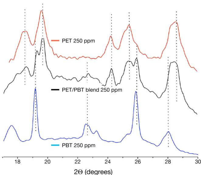
Figure 4. WAXS of PET, PBT and PET/PBT blend with 250ppm of catalyst.
