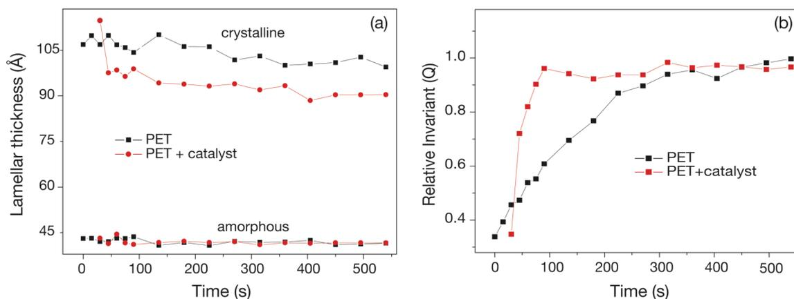
Figure 2. Time evolution of the crystalline parameters of the PET with and without catalyst during the crystallization at 210 °C.
