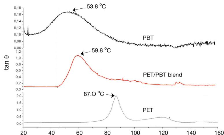
Figure 6. DMTA curves for the PBT, PET and PET/PBT blend.
