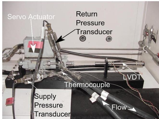
Figure 7. The servo actuator experiment.
