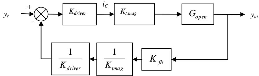
Figure 6. Servo actuator model diagram for identification.
