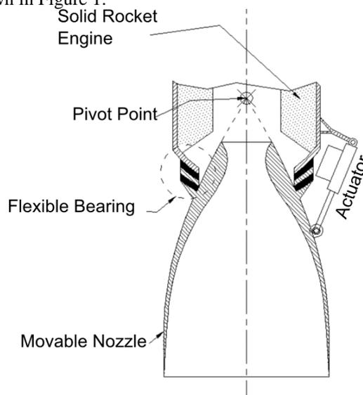
Figure 1. Scheme of thrust vector control by movable nozzle.
