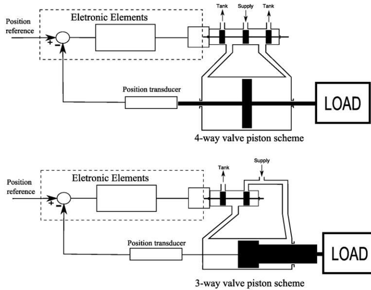
Figure 2. General three-way and four-way valve piston schemes.
