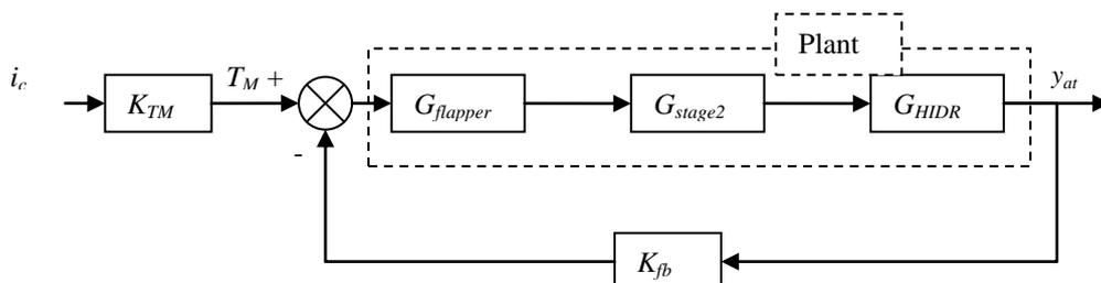
Figure 4. Proposed model structure for the servo actuator.
