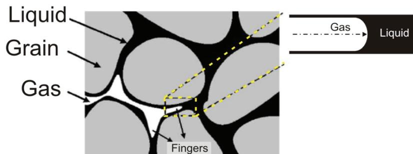
Figure 1. Representation of relationship between capillary tube and porous medium approach.
