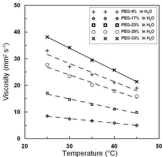
Figure 3. Behavior of kinematic viscosity increasing fluid temperature.
