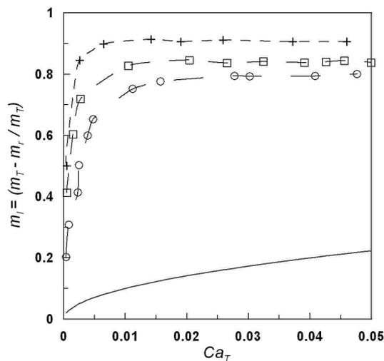
Figure 5. Mass lost versus Taylor Capillary number. Particles ranges: Dashed line with (+ +) is to 500-900  $\mu m$ , with ( $\square \square$ ) is to 1000-1400  $\mu m$  and with ( $\circ \circ$ ) is to 1400-2000  $\mu m$ . The continuous line (—) is to show the Taylor curve reference.
