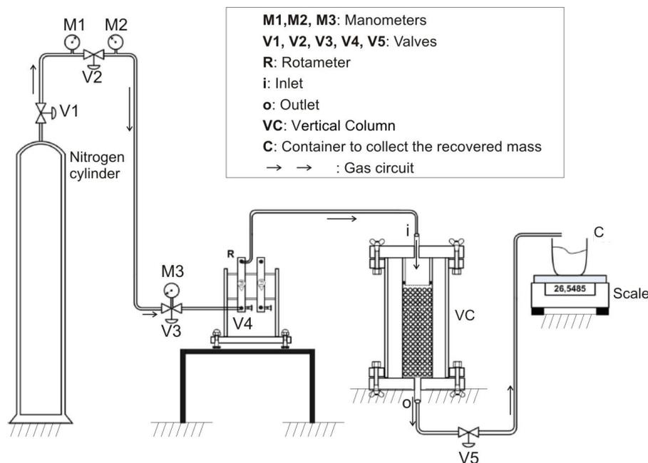
Figure 4. Experimental setup
