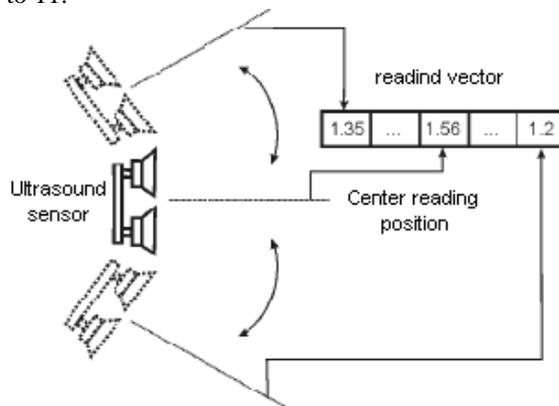
Figure 9 – Reading procedure of the side sonar.
