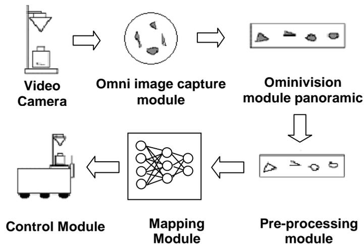
Figure 5. Processing stages of the LACE mobile robot omni vision system
