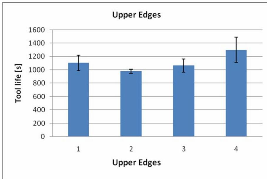
Figure 4. Average tool life for each upper edges of the square insert
