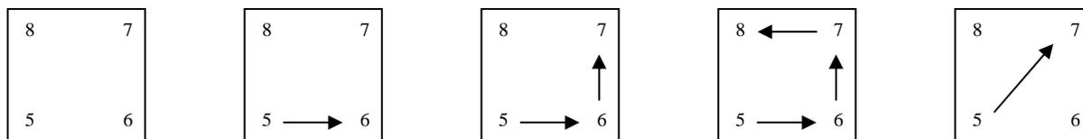
Figure 3. Sequence for testing the bottom edges of the square cemented carbide insert
