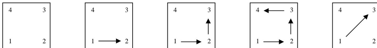
Figure 2. Sequence for testing the upper edges of the square cemented carbide insert
