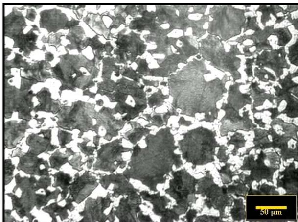
Figure 1. Micrography of the DIN 38MnSiVS5 HSLA steel used in the tests (etched with 2% Nital)
