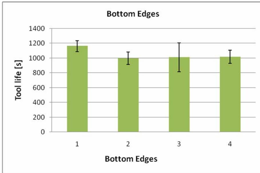
Figure 5. Average tool life for each bottom edges of the square insert
