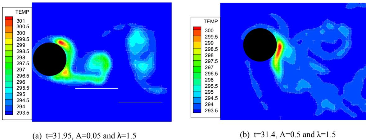
Figure 4. Temperature distributions at B point for transverse oscillating circular cylinder case,  $Re=1.0 \times 10^5$  and  $Pr=0.71$ .
