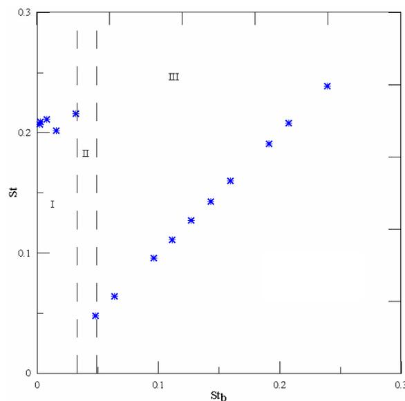
Figure 2. Circular cylinder: frequency of vortex shedding,  $A/d = 0.50$  and  $Re=1.0 \times 10^5$ .
