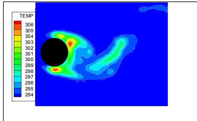
Figure 6. Temperature distributions at B point for fixed circular cylinder case,  $Re=1.0 \times 10^5$  and  $Pr=0.71$ .
