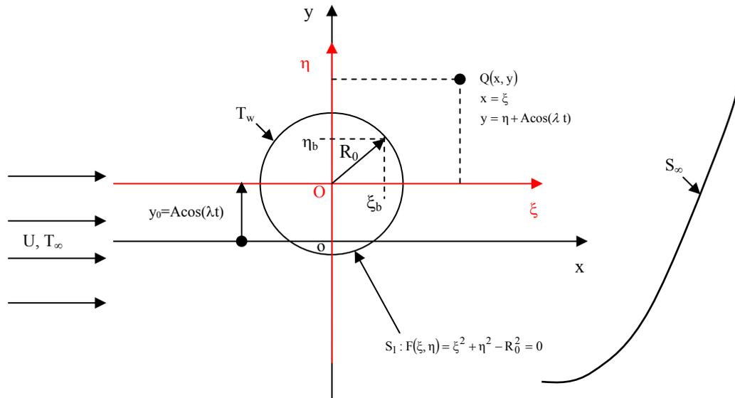
Figure 1. Transversely oscillating heated circular cylinder in uniform freestream flow.
