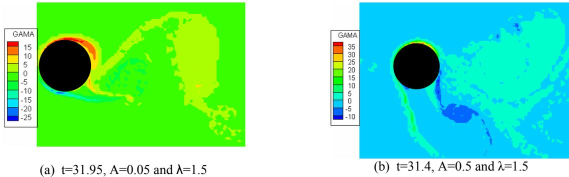
Figure 5. Vorticity field at B point for transverse oscillating circular cylinder case,  $Re=1.0 \times 10^5$  and  $Pr=0.71$ .
