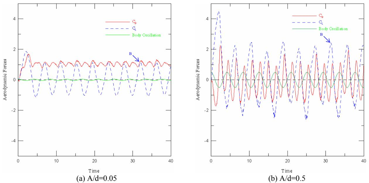
Figure 3. Variation of  $C_D$  and  $C_L$  with time,  $\lambda=1.5$  and  $Re=1.0 \times 10^5$ .
