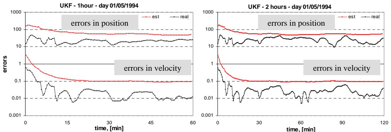
Figure 4. Errors in position and in velocity for the 1 and 2 hours, respectively, through UKF-EKF
