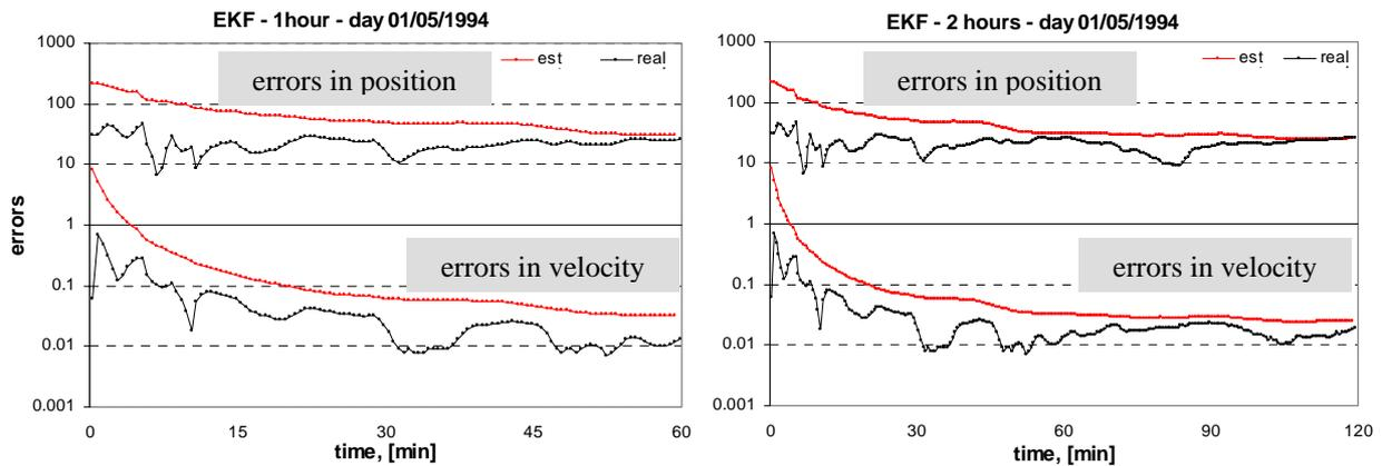
Figure 6. Errors in position and in velocity for the 1 and 2 hours, respectively, through EKF
