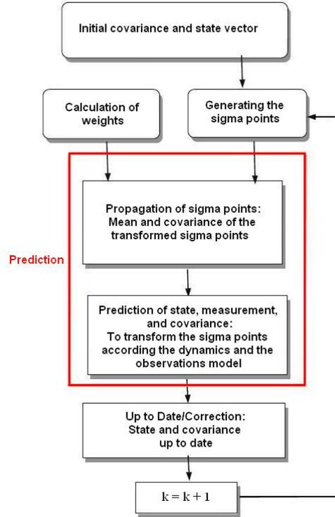
Figure 1. Modified Kalman Filter, leading to UKF
