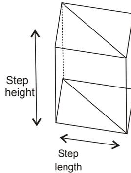
Figure 3. Detail of the dimension of a stair step.
