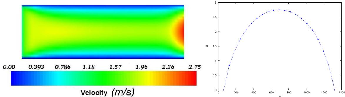
Figure 4. Simulation at a domain with stairs, field of velocity component in direction  $x$  with  $Re = 10$ , with five layer of prisms.
