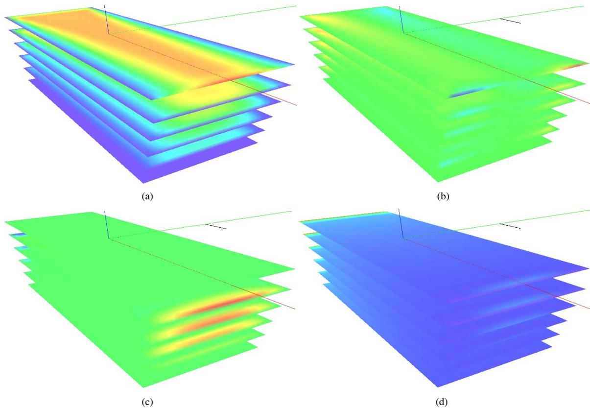
Figure 7. Numerical simulation of the flow with stair on domain: a) Field of velocity component at direction  $x$ , b) Field of velocity component at direction  $y$ , c) Field of velocity component at direction  $z$  e d) Pressure profile using  $Re = 100$ .
