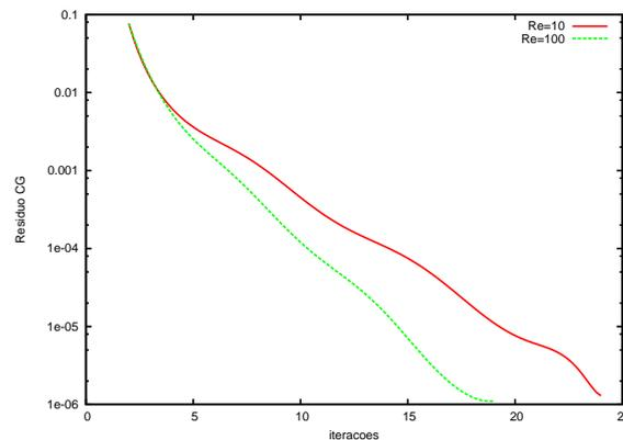
Figure 6. Residue of the conjugate gradient method over the iterations.
