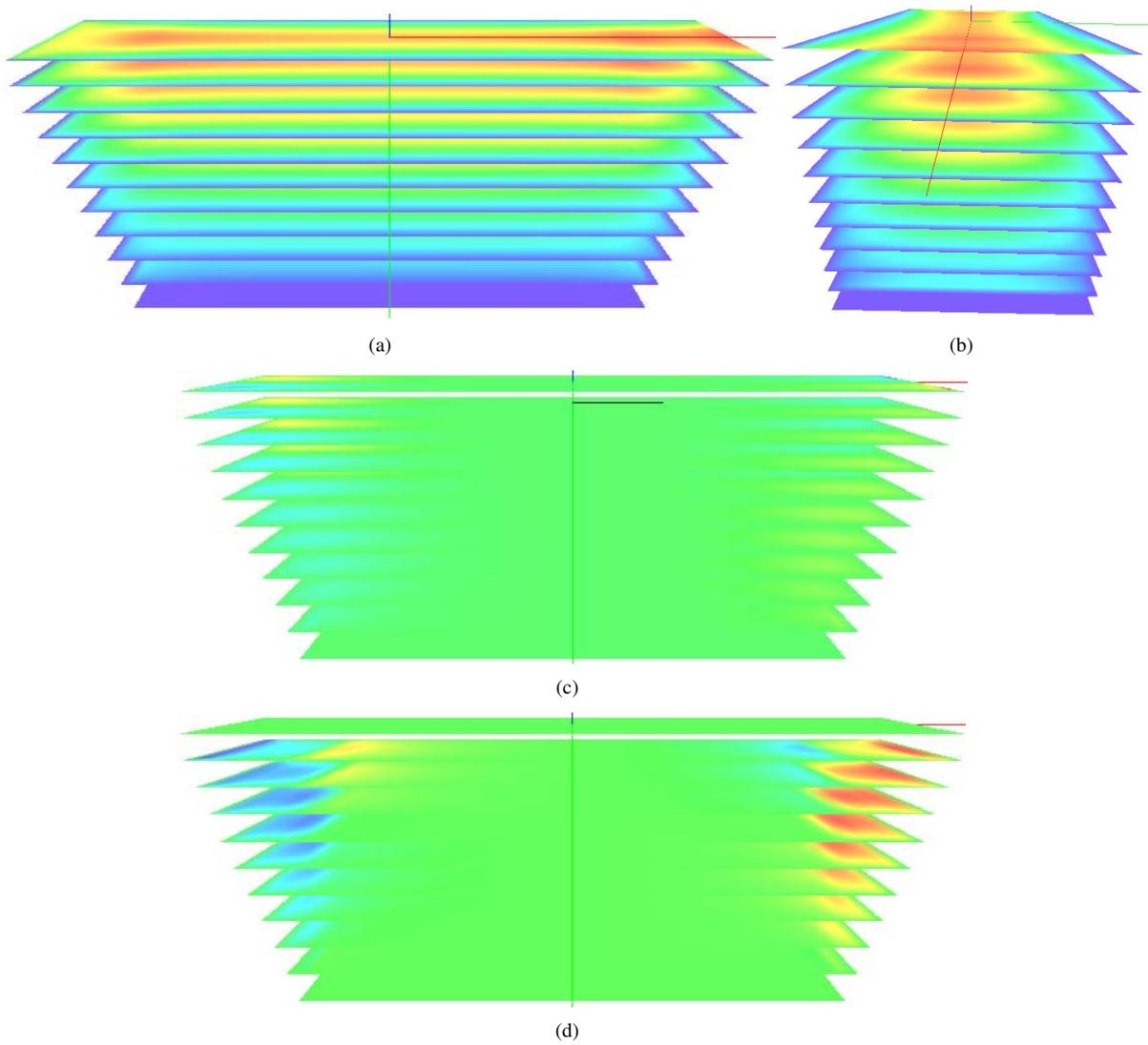
Figure 8. Numerical simulation of the flow with stair on domain: a) Field of velocity component at direction  $x$ , b) Field of velocity component at direction  $y$ , c) Field of velocity component at direction  $z$  e d) Pressure profile using  $Re = 1$ .
