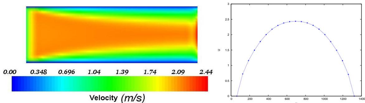
Figure 5. Simulation in a stair steps domain, field of velocity component in direction  $x$  with  $Re = 100$ , with five layer of prisms.
