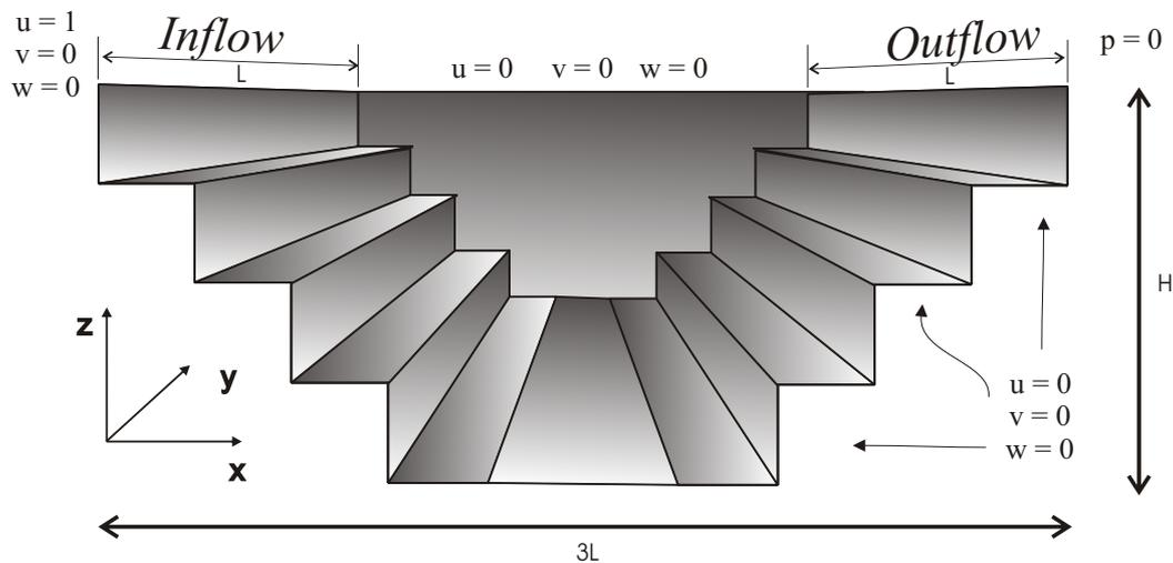
Figure 2. Perspective on  $y$  axis e boundary conditions for the simulation using stairs on reservoirs.
