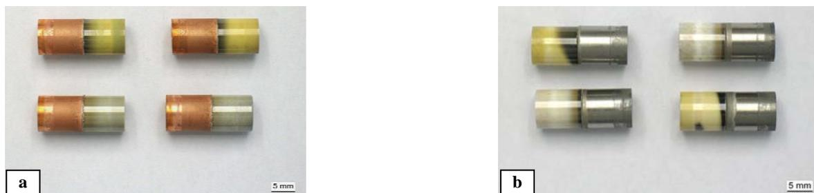
Figure 8. (a)  $ZrO_2/Ag-28Cu/Cu$  joints; (b)  $ZrO_2/Ag-28Cu/Ti-6Al-4V$  joints. Darkening effect in zirconia localized from the joint interface for brazing tests at  $820^\circ C$  (TZP-Y in white and PSZ-Mg in orange color).
