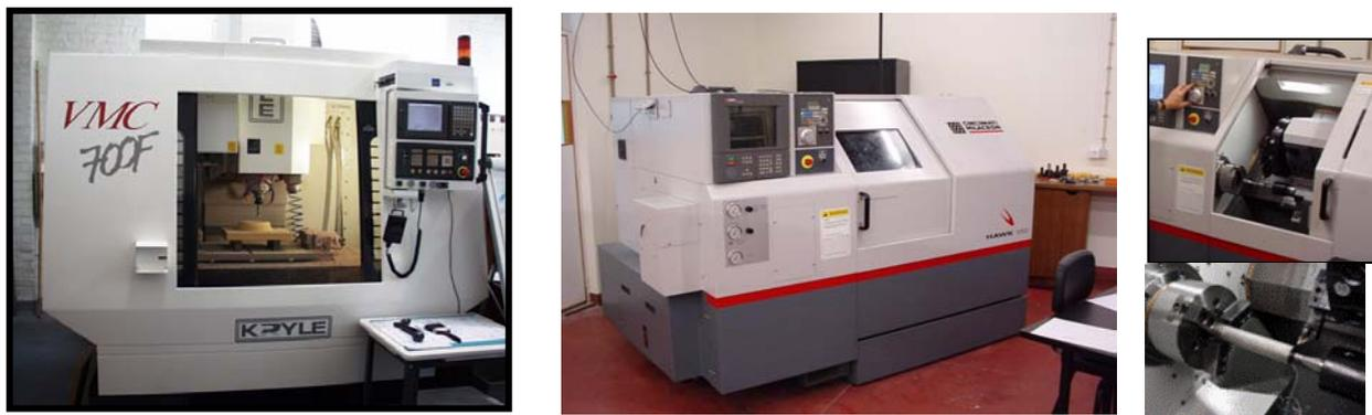
Figure 5. Modern CNC machines accept numerical instructions to control its moving elements;
