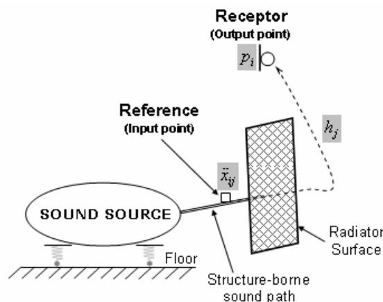
Figure 1. Illustration of the operational TPA methodology considering one source and one structure-borne sound path
