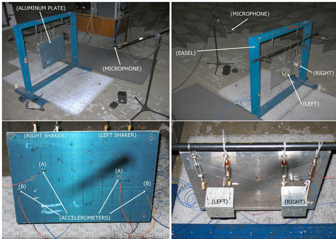
Figure 2. Set-up (A) and (B) for the TPA validation using a semi-anechoic chamber
