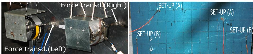
Figure 3. Force transducer and accelerometer positioning in detail for set-up (A) and (B)
