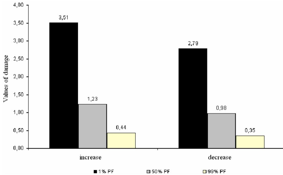
Figure 5. Values of the damage - theory of Palmgren-Miner.
