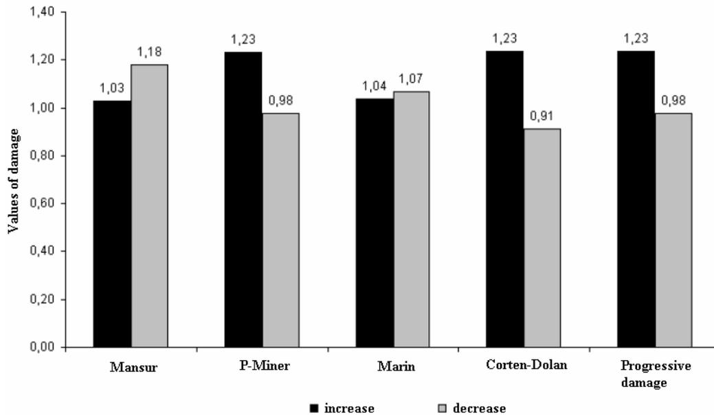
Figure 11. Comparison of the theories for a failure probability of 50%.
