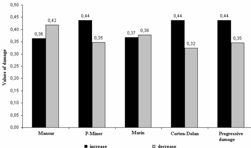
Figure 12. Comparison of the theories for a failure probability of 99%.
