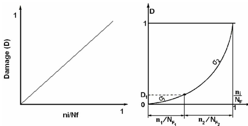
Figure 2. Linear and not linear model damage
