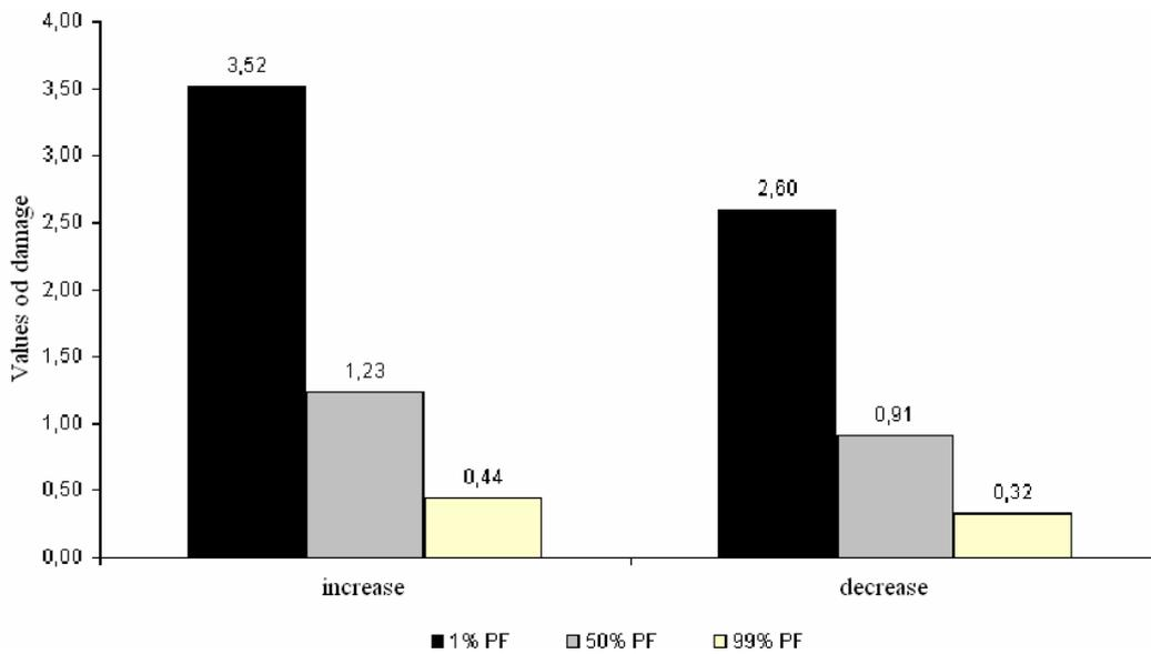
Figure 6. Values of the damage - theory of Corten-Dolan.
