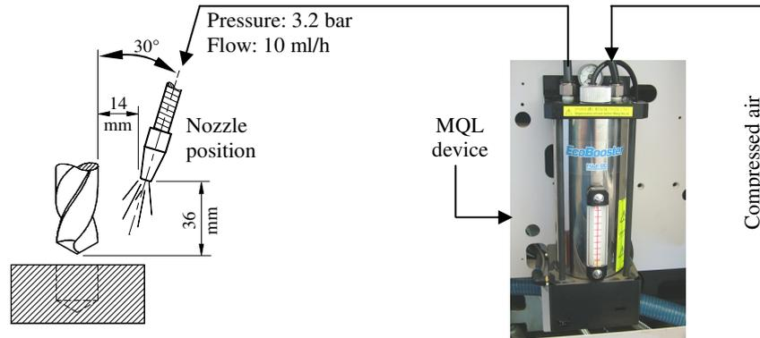
Figure 3. MQL device and external nozzle position.
