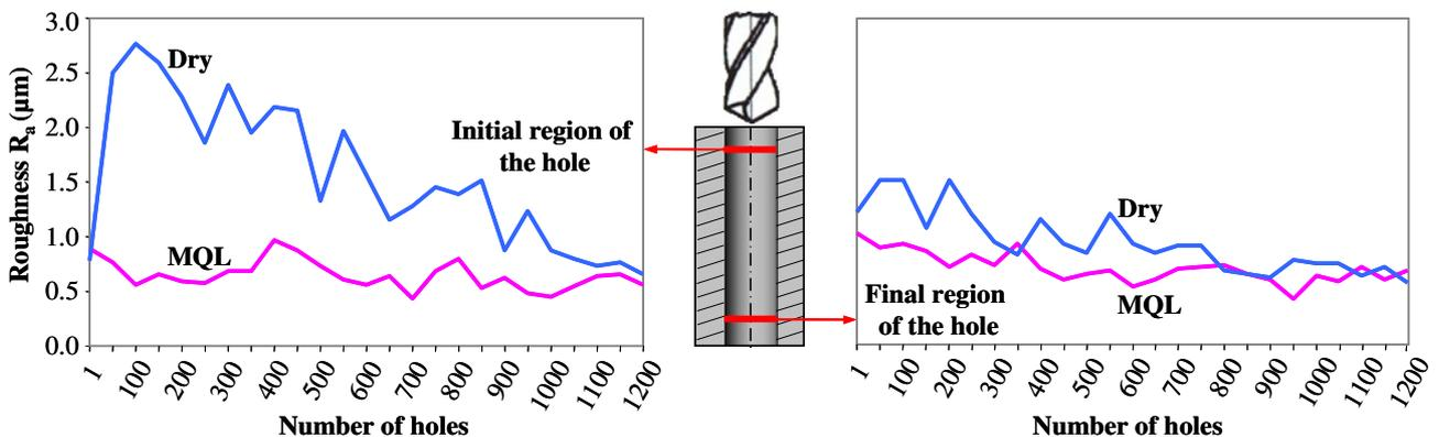
Figure 4. Graphs of roughness  $R_a$  values measured in the initial and final regions of the holes.
