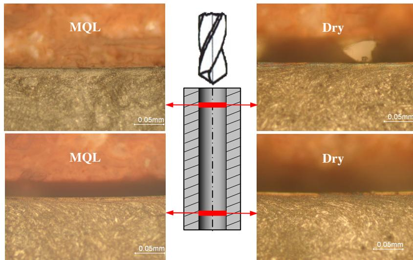
Figure 7. Typical region of plastic deformations in the initial and final regions of the  $1200^\circ$  hole.
