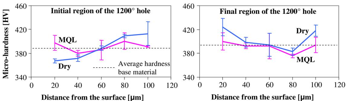
Figure 8. Graphs of the surface micro-hardness versus the distance from machined surface.
