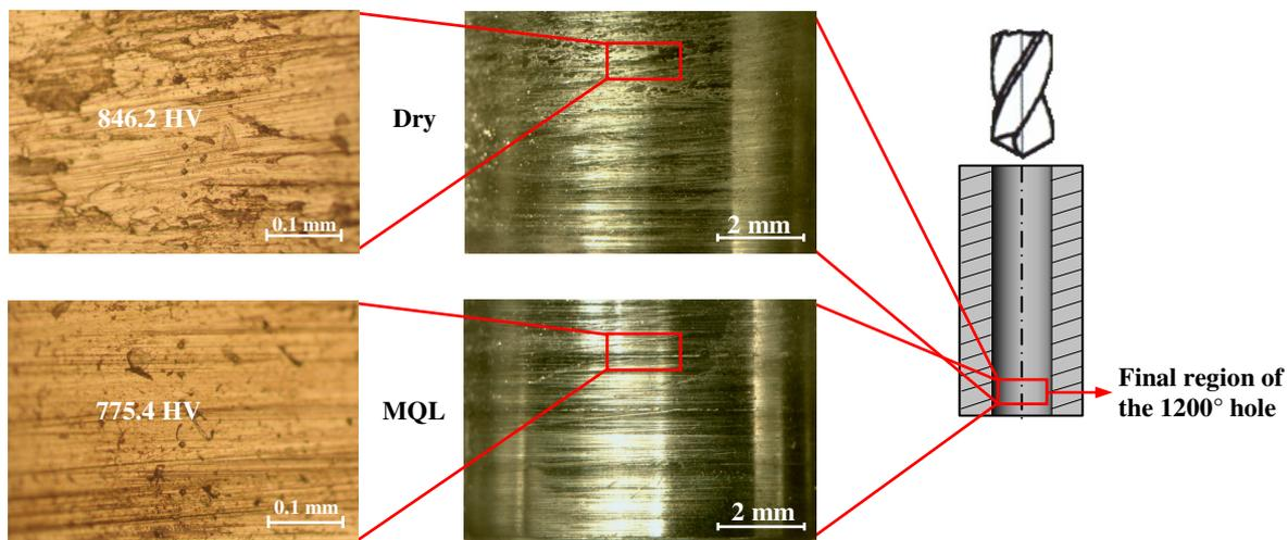
Figure 5. Surface texture at the end of the last holes.
