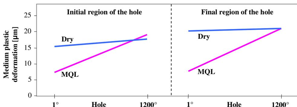
Figure 6. Medium plastic deformation in the initial and final regions of the holes.
