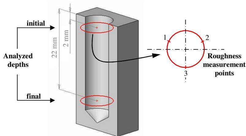
Figure 2. Analyzed depths and roughness measurement positions.
