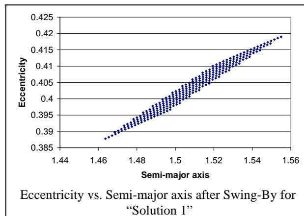
Fig. 2(b) – Swing-by for a cloud of particles with Jupiter for  $r_p = 1.1 R_J$
