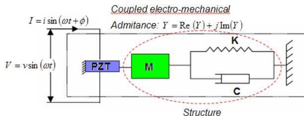
Figure 1: One-dimensional model used to represent a PZT patch-driven dynamic structural system.
